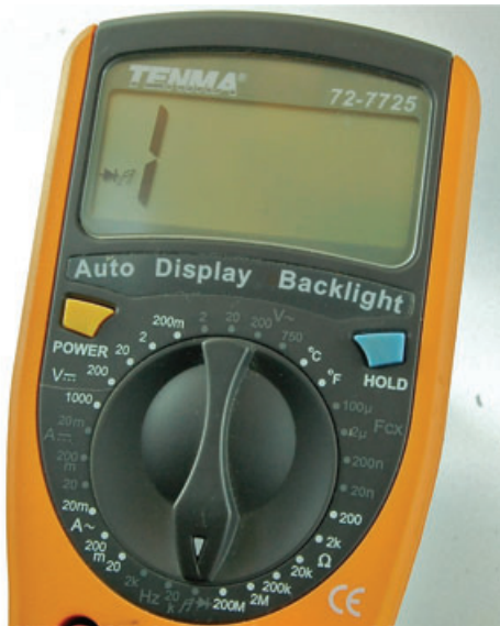
FIGURE 1-8 A multimeter in Continuity mode
