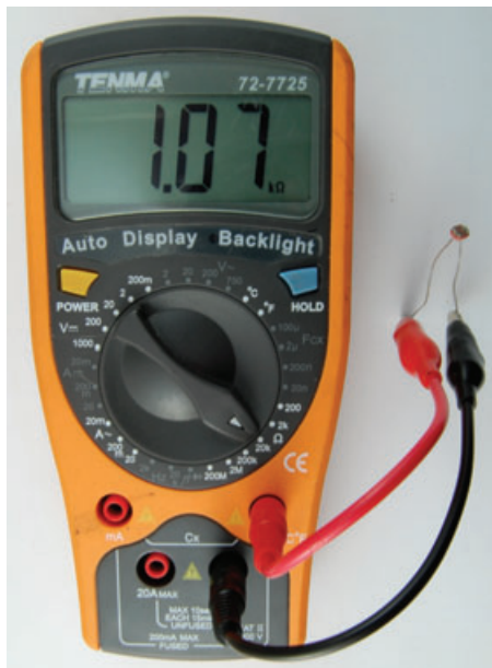
FIGURE 3-8 Measuring the LDR resistance
