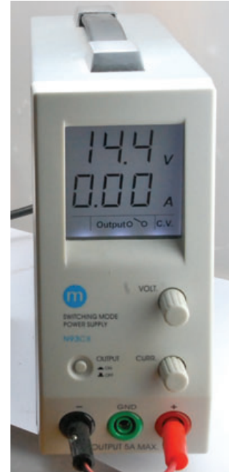
FIGURE 11-7 A lab power supply
