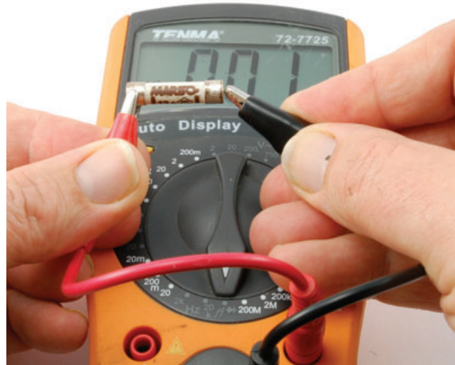
FIGURE 10-3 Testing a fuse with a multimeter
