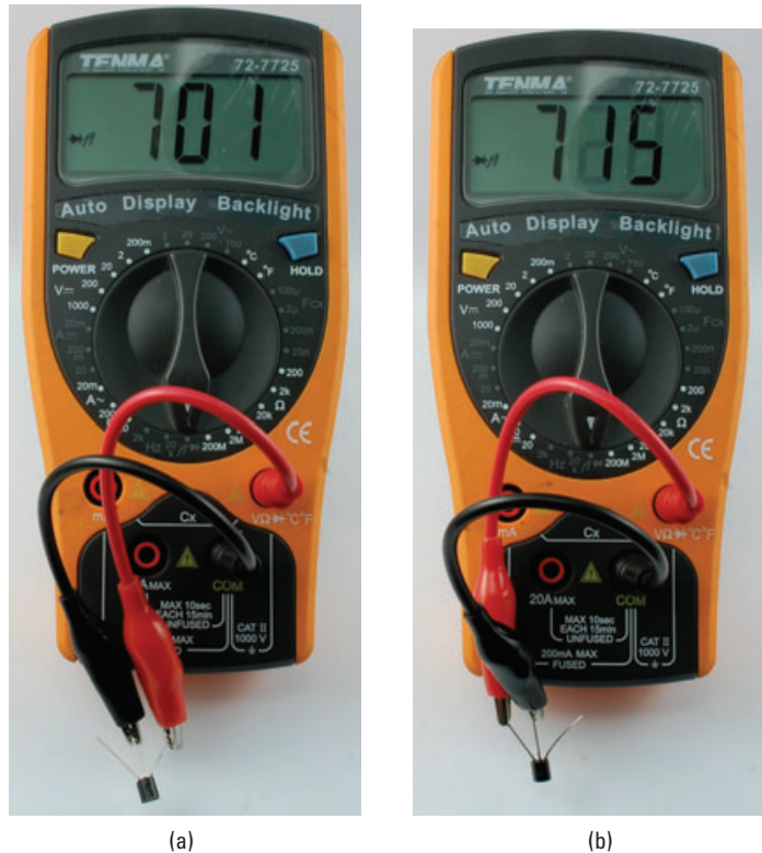
FIGURE 11-6 Testing a transistor
