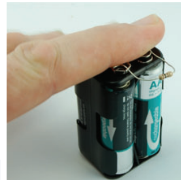
FIGURE 3-3 Making a resistor get hot
