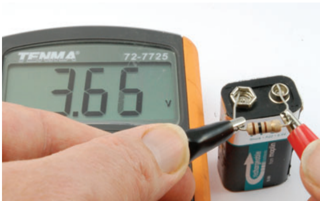
FIGURE 10-4 Testing a battery using a resistor and multimeter
