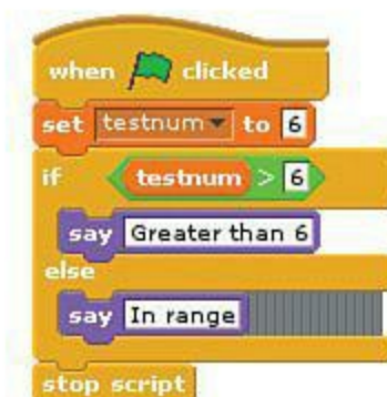
FIGURE 8.1 A conditional logic expression in C (top) and in Scratch (bottom).
