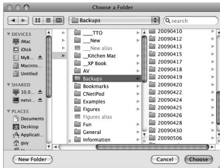
Figure 8-23 Without any parameters, the Choose A Folder dialog box displays no prompt and hides invisible folders.
