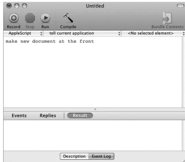
Figure 3-2 You can place the Tell Application pop-up menu in the navigation bar by selecting the Show “Tell” Application Pop-Up Menu in Editing preferences.
