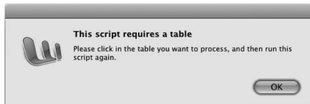
Figure 14-4 If checking reveals the selection to be of the wrong type, you can tell the user which type of selection is needed.
