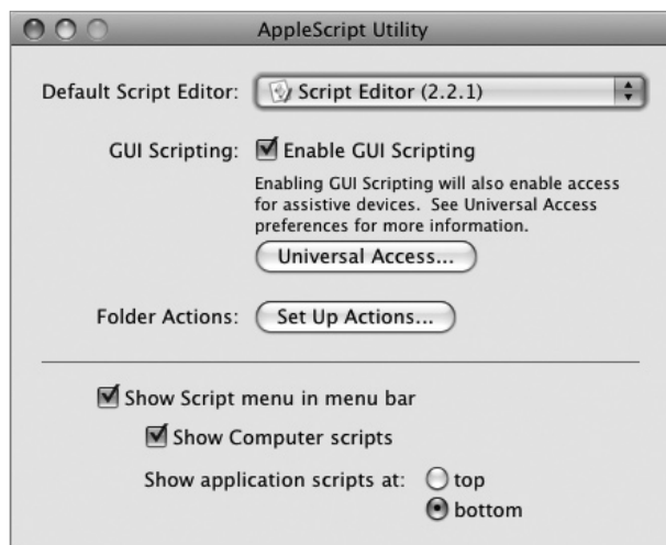
Figure 2-8 AppleScript Utility lets you control whether the Script menu appears on the menu bar in Leopard and earlier versions of Mac OS X.
