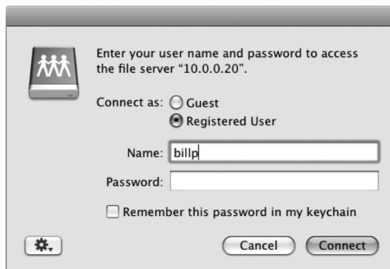
Figure 6-1 If you don't include the password when mounting a volume, the user has the choice of entering the password or trying to connect as a guest user.
