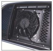
Heavy-Duty Exhaust Fan quickly circulates air inside the car (KK-K9-FKT-I mounted on KK-K9-FAN-F7-1-OBR)
