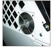
**Circulation Fan** draws AC/ heat into rear compartment (KK-K9-FAN)
