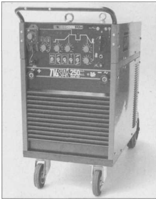
6.12 When you go up in welding machine size, you get more amperage and higher duty cycles. This TIG-Star 250 operates on several single-phase input currents, and has a 60% duty-cycle at 200 amps, with 100% duty-cycle at 140 amps.
