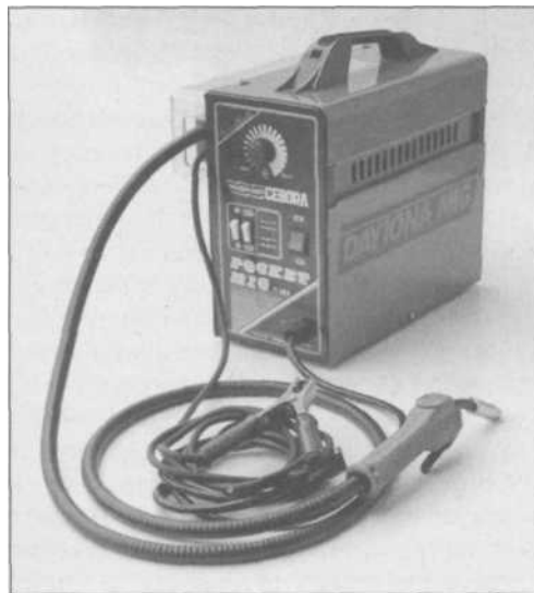
5.16 A popular entry-level MIG machine is this 110-V Pocket-MIG from Daytona MIG. Though it weighs only 42 pounds, it has an amp range from 30-110 amps, capable of welding up to 1/4-inch steel. Very portable, it's ideal for home/shop use, especially on sheet metal.
