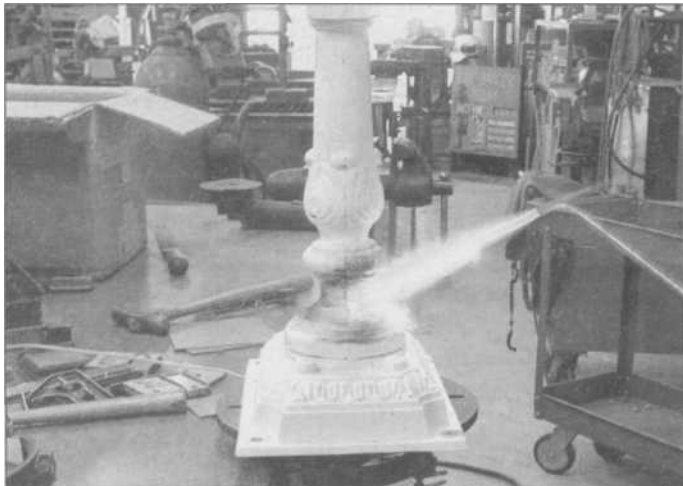
3.54 The rosebud tip will be useful for heating metal parts to be bent, freeing press-fitted parts, and for preheating castings before welding, such as here where a cast-aluminum mailbox post is preheated before TIG welding.
