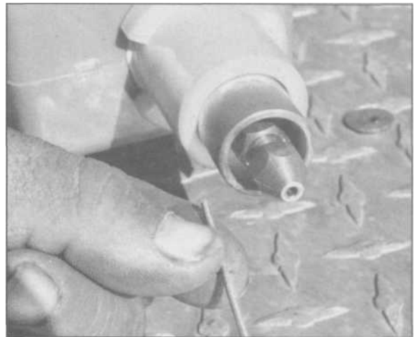
8.34 Small-headed copper-plated "studs" are inserted into the magnetic head of the stud setter.
