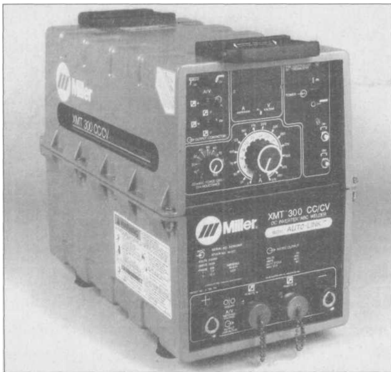
4.7 In larger welding shops, a more sophisticated power source is used, such as this 300-amp Miller DC machine, which has a few more "bells and whistles" than the home-type units.
