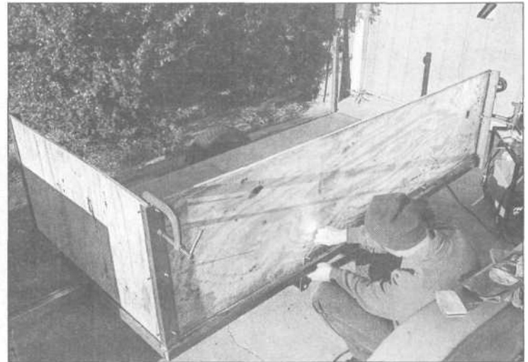
9.31 Plywood sides are bolted to the end pillars and the side plates.
