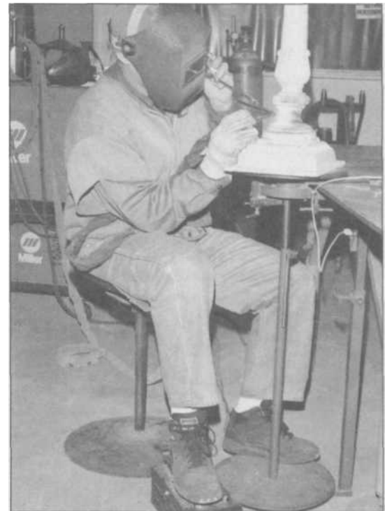
6.36 Weldor Bill Maguire is TIG-welding the heated mailbox post, using his rotating welding stand he invented. At the bottom is a round disc you can spin with your foot, leaving your hands free to continue welding, especially where you have to go around something. These should be available for sale at the time of printing.
