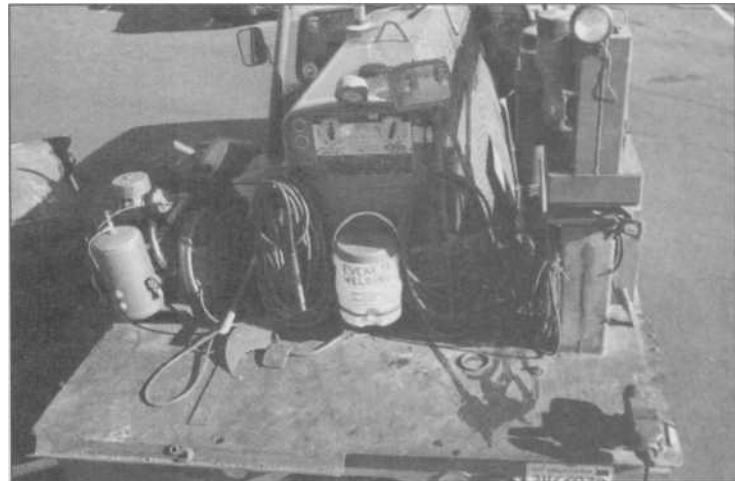
1.12 The back of the same oil field welding truck is built as a large, heavy workbench-away-from-a-shop. Big Lincoln ac/dc arc welder has its own engine power and generator to run lights for night work.
