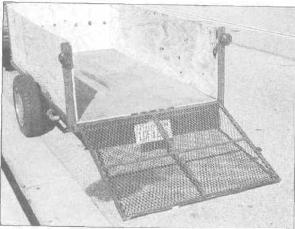
9.37 With the wingnuts undone, the hinged tailgate folds down as a ramp for furniture dollies, lawnmowers, etc. The trailer should be hooked up to the tow vehicle before you step on the tailgate/ramp, or the lightweight trailer could tilt quickly.
