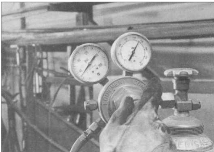
3.20 Gas flow is regulated on the oxygen cylinder to 1-5 psi for welding, depending on the thickness of the material to be welded, and the acetylene pressure is adjusted the same. Higher pressures are set when performing cutting, but acetylene must never exceed 15 psi to the torch.
