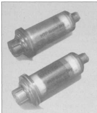
7.27 Dry, clean shop air is extremely important to extending the life of your plasma nozzles and electrodes. These HTP Super-Dry air driers have a bronze filter and desiccant inside that changes color when it needs to be changed.
