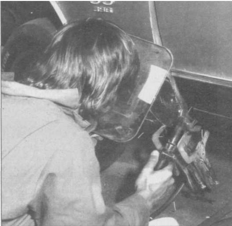
5.55 Don' be tempted by the low spatter of MIG welding to just shut your eyes when tacking body panels. If you need speed and convenience while tacking, use a hand-held safety-shield with lens as shown here. Weldor here has long sleeves, but should have gloves on and a turned-around hat to protect his hair from hot spatter.
