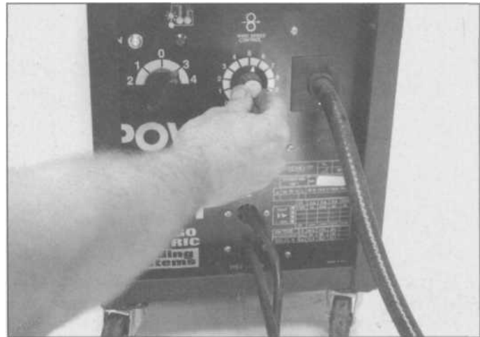
5.41 The wire speed has a lot to do with the heat and quality of the weld. Generally when you have it right, the MIG machine makes a very satisfying steady "sizzle" sound. Practice by adjusting the feed high and gradually lowering it until the sound and results are satisfactory. If you do repetitive projects, write down the amperage and wire speed settings that have worked for you.
