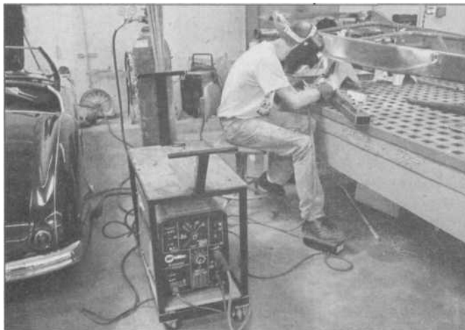
6.24 The pedal is the final weldor control of the amperage in TIG welding. Until you are experienced, you may want to set the amperage knob at the highest you need for a particular job, and know that when you are welding, the pedal can go all the way. It takes some experience to know how much pedal to give, if the knob is set to the max for the amp range on the coarse adjustment.
