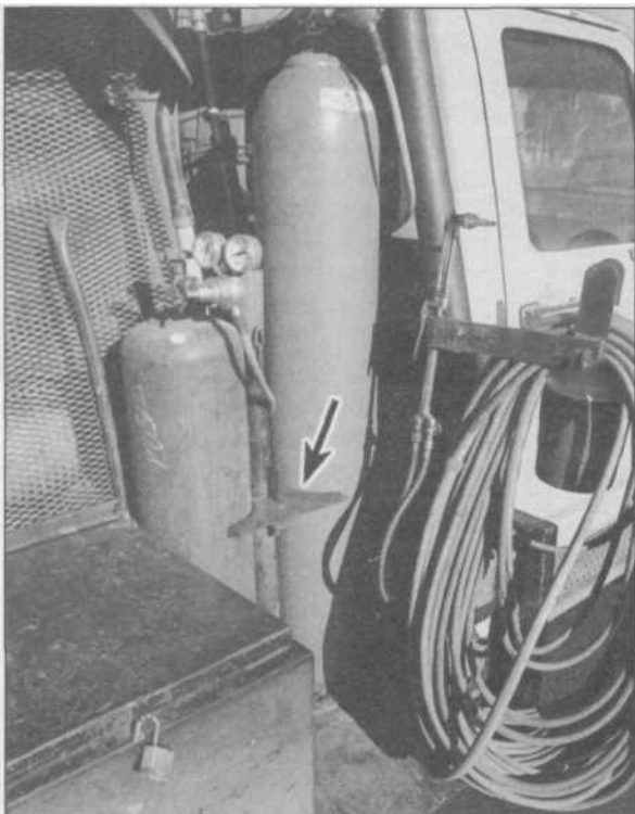
3.13 In this clever setup, the hoses and torch are attached to a swingaway arm for access to the tanks for servicing. Arrow indicates retaining plate with a simple steel wedge rod. Tanks are held securely but can be changed quickly without wrenches.
