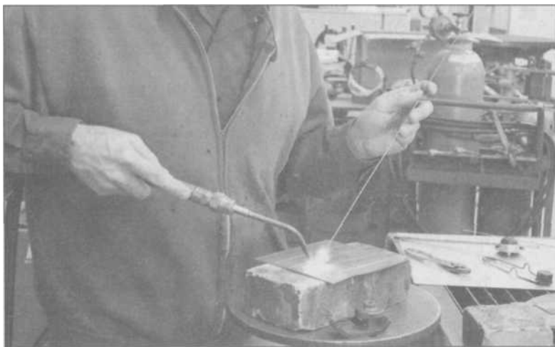
3.24 You don't have to worry about grounding with gas equipment, but there is a dangerous flame involved, so your welding projects and practice sessions are best done over some firebricks like this, which you can get at your welding supply store.
