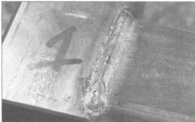
Small heat-affected zone on MIG weld
