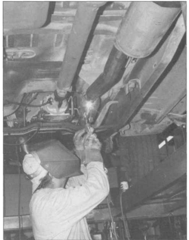
5.59 Muffler shops are finding that the MIG machine is faster and safer to operate under a car than the traditional oxy-acetylene torch equipment. There is no constant re-lighting and adjusting of the flame to worry about when initially tack-welding various pipe sections together.
