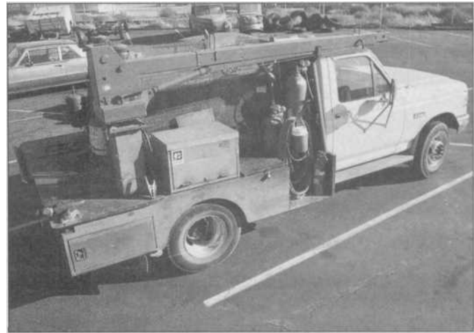
1.11 Not every welder and weldor works indoors. This is an oil field service truck with gas-welding/cutting equipment, arc welder and crane. Many welding shops have portable setups like this for remote jobs.
