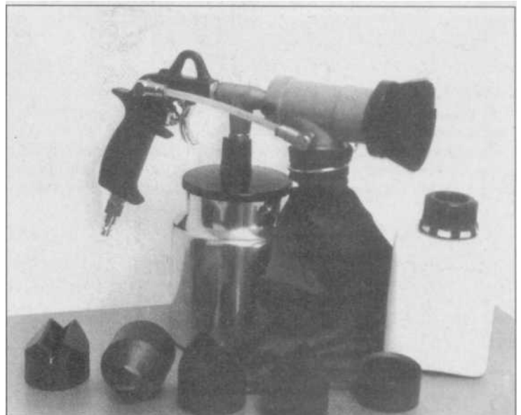
8.47 Daytona MIG sells this handy spot-sandblaster. It is useful for cleaning paint and rust away from a spot you have to weld, like a recess where a regular sander won't reach. Three-quarters of the blasting media is returned to the gun, so it won't make your shop a "sandpit."
