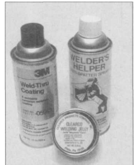
5.13 These three chemicals are helpful in performing clean welds and maintaining your MIG torch in good condition. The anti-spatter spray and gel are used on the nozzle to make removal of debris easier, and the weld-through coating by 3M is used when welding high-strength steel in late-model cars. Unlike the other sprays, it is applied to the area to be welded, providing extra corrosion protection after the weld.
