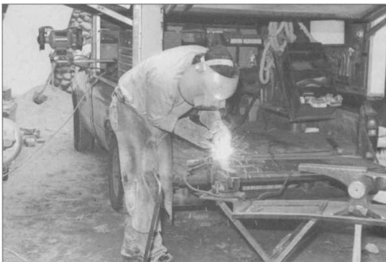
1.3 The farrier of today works out of a truck, filled with equipment like a grinder, drill press and welder, all running on AC power when available; otherwise, horseshoes are shaped in a portable forge. Today's blacksmith has the advantage of tools like this MIG welder that speed up making special horseshoes.
