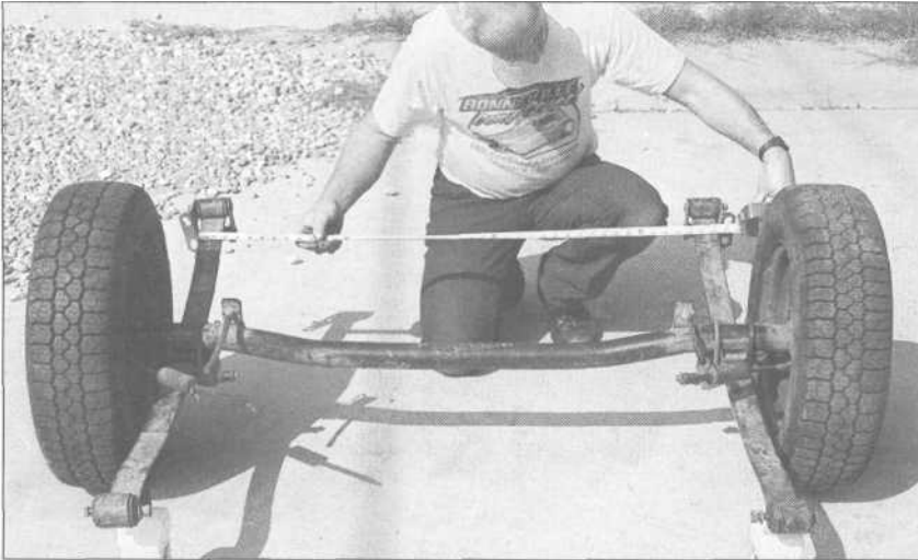
9.6 In our case, we determined that the Sprint axle was too narrow for our purposes, since we wanted a full 4x8-foot sheet of plywood as a floor. This meant widening our tubular axle 7 inches.
