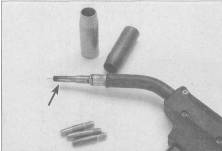
5.9 Most MIG nozzles just twist off past a snap ring, exposing the contact tube (arrow). You should keep an extra nozzle as a spare, and several spares of the sizes of contact tubes (below) that you use most. Eventually, you will weld the wire to the contact tube, and have to unscrew it to get it off, then clip off the wire and install a new tube, also called a contact tip.
