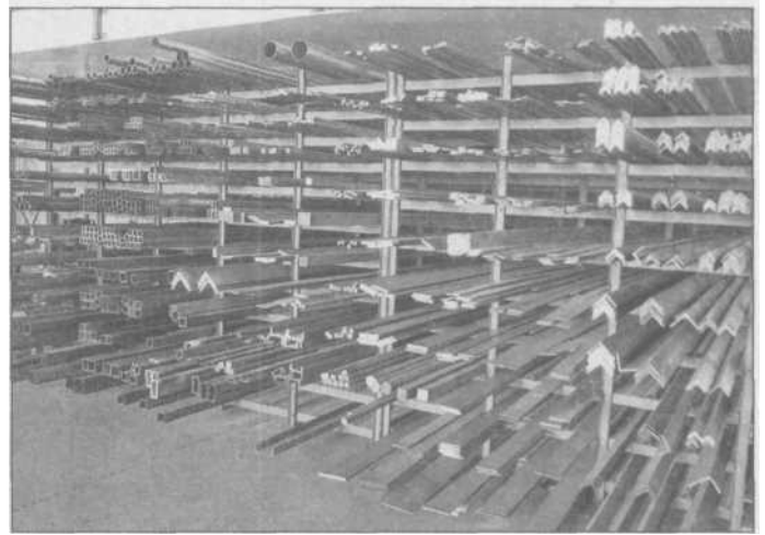
2.31 This steel supply store has a neatly-organized rack for materials, in which each different thickness of material is identified by a different color of paint on the ends, which makes shopping a lot easier for hobbyists without a micrometer.
