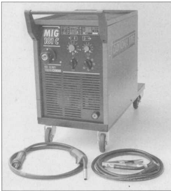
5.23 This 220V unit, the 181C from Daytona MIG, offers settings from 20 amps for light sheet metal to 180 amps for heavier work, and has a spot-timer and quick-disconnect torch. This is suitable for light fabrication shops.
