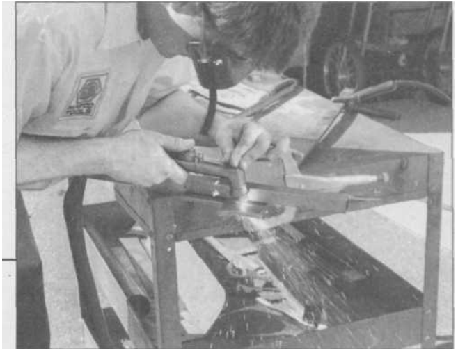
7.1 Plasma cutting can be done outdoors, being very little bothered by wind, makes very clean cuts on ferrous and non-ferrous materials, and produces no smoke and very little sparks. It has become the modern way to cut metal. The operator here should be wearing gloves and a long-sleeved shirt.
