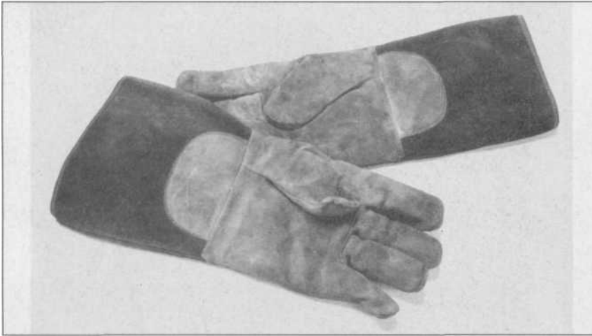
8.8 A good pair of leather welding gloves will last you for many years, but if you are using oxy-acetylene equipment, keep an extra-clean pair for use with this equipment. A spurt of oxygen on a dirty glove could cause combustion, so don't use these good gloves for handling hot or dirty parts.
