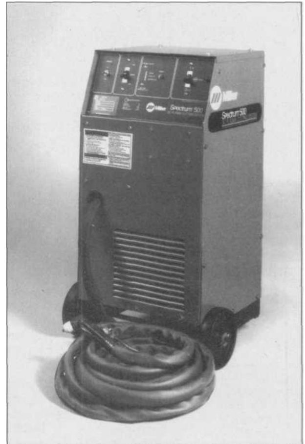
2.27 In fabricating shops, a large 220V (or higher current, three-phase) plasma cutter is used, capable of cutting thick materials and traveling at fast cutting speeds. Most plasma cutters are used without shielding gas, using air from the shop air compressor to cool the torch and form the ionized gas column under the tip that creates the arc.
