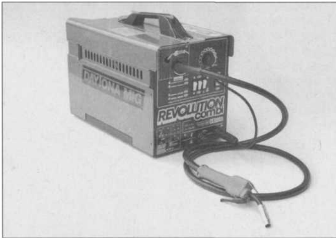
5.18 If you need the flexibility of welding indoors and out, a combination MIG that uses either gas-shielding or flux-cored wire fills the bill. This Combi 888 runs on 110V power, with 130-amp capacity.
