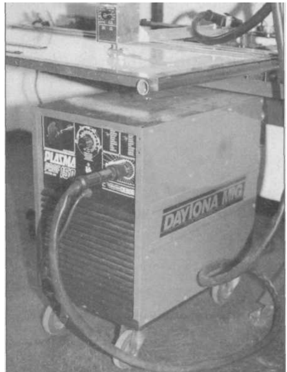
7.12 The bigger-amperage machines are all in the 220V category, and many, like this Daytona MIG Plasma Prof 50, require shop-type three-phase current, too. This one has a 35% duty-cycle at its rated max of 50 amps and 100% at 30 amps.
