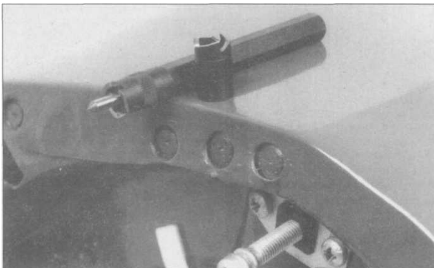
8.20 For Eastwood offers a similar tool for removing spot welds which features a hex-sided drive end, so it can't slip in your drill chuck.
