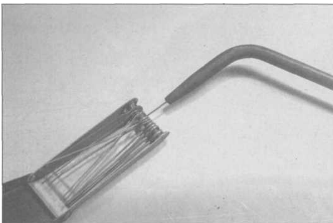
3.29 As you weld, it is inevitable that sparks and spatter will blow back onto your torch tip. If it plugs up, your bead will be spotty and your torch may go out entirely. Keep the tips clean with a set of fine-wire cleaners that come with your gas set.
