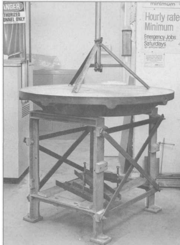
8.22 You never know when you'll find something that comes in handy in the shop. This huge and hefty round plate was found at a metal yard and bought at the per-pound price. It's dead flat and cannot warp, and has mounting holes in it for clamping work to it.
