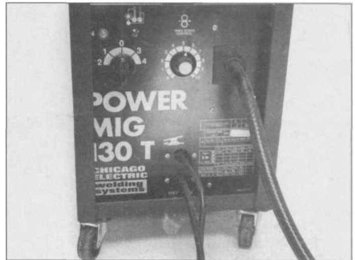
5.6 There are very few user controls on the panel of a basic MIG welder, just a switch for the different amperage settings, and a variable knob for controlling the wire-feed speed.
