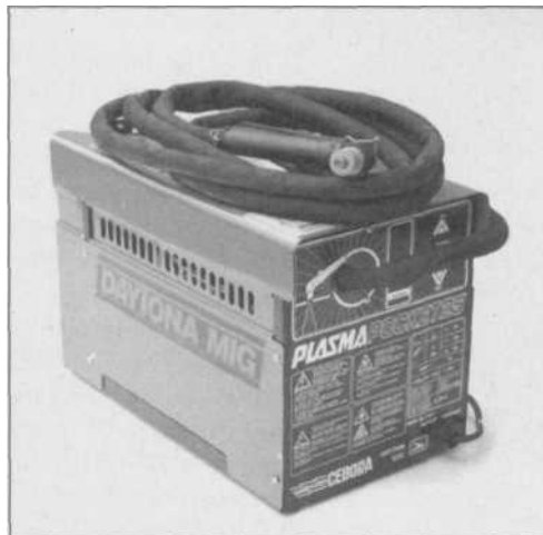
7.7 The compact end of the plasma cutter market is represented by 110V machines such as this Plasma Pocket from Daytona MIG. It puts out 25 amps, weighs 55 pounds, and requires 4-6 cfm of air at 70 psi.
