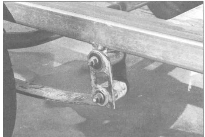
9.23 After some solid tack-welding, pull the springs out so the bushings don't melt, and fully-weld the four front spring mounts. Here the springs are bolted back in.
