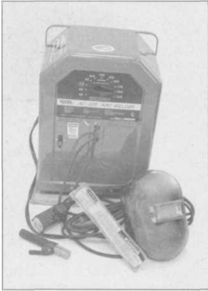
4.2 For home and farm use, the Lincoln 225 is the classic AC buzz-box welder, having been in production relatively unchanged for decades. Most home/shop units are AC only, and require some rewiring to accommodate the required 220V input.
