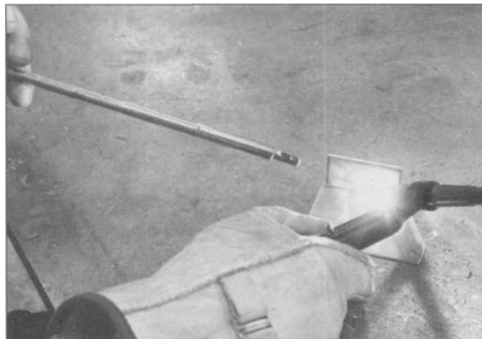
6.33 When you are learning TIG welding on aluminum, keep your torch angle so that you can get a good, close look at how the puddle develops and the molten area becomes shiny. You need enough heat to form the puddle, but not much more or the aluminum vaporizes.
