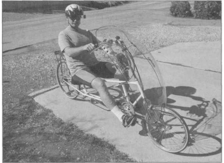
2.6 Welder Bill Maguire fabricated this recumbent bicycle for himself from 4130 chrome-moly thinwall tubing, which is very strong but light. The idea was to reduce the bike weight, wind resistance and pedal effort. Bill joined the thin tubing with TIG welding.
