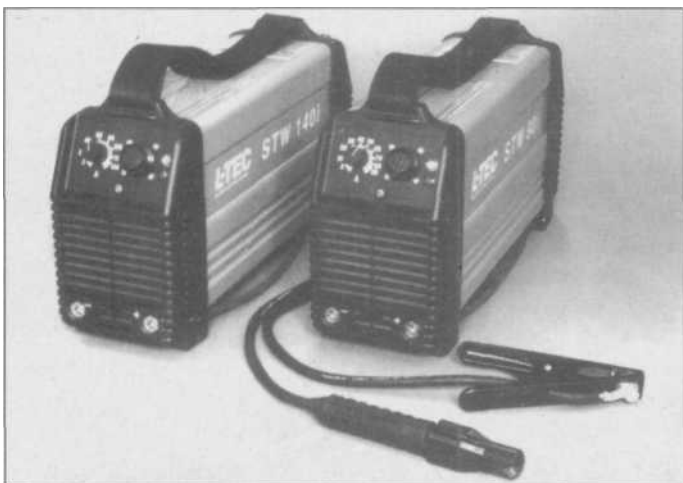
4.29 These L-TEC portable arc power sources are lightweight, and offer up to 90 amps on the STW 90i (right) and 130 amps on the STW 140i. Unlike most small arc welders, these are DC, and can even be set up with a torch and power adapter to run a TIG torch. They are available for 110V or 220V input.
