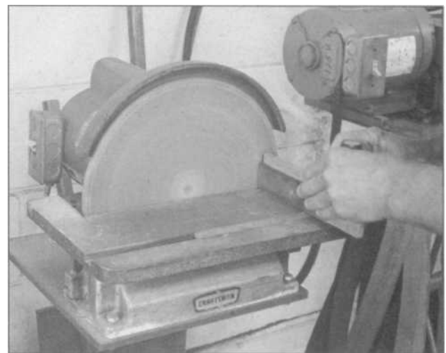
8.24 A disc sander with at least 1/2 horsepower is very handy around the shop for squaring edges of flamecut parts, and taking sharp edges and corners off work.
