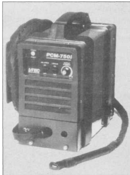
7.13 Still light and portable, but powerful enough to cut 3/4-inch steel, The L-TEC PCM-750i has 50 amps with a 40% duty-cycle at that setting, and has its own torch storage spool and spare parts storage compartment.
