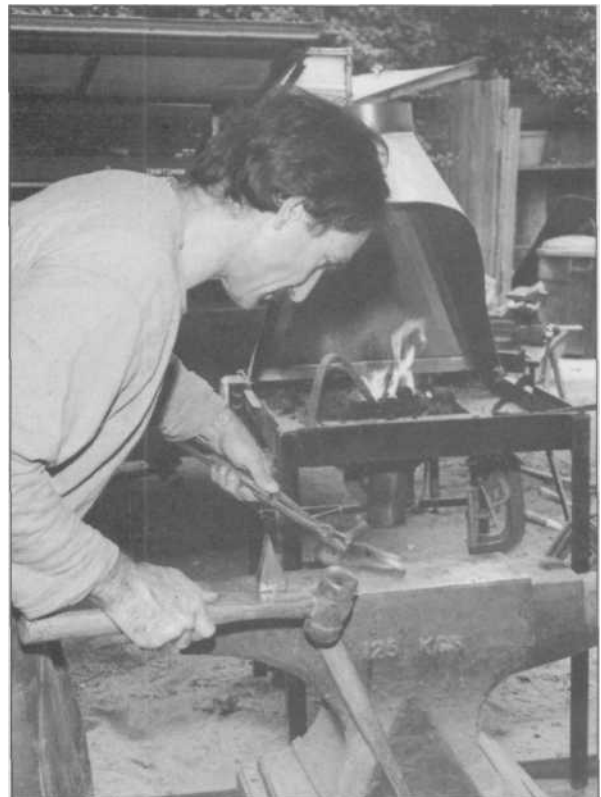
1.1 Welding had its ancient origins in the fires of blacksmiths, who could forge two white-hot pieces of metal together with hammer blows and patience. It remained for history to bring us to electricity and bottled gasses for welding techniques to develop any further. Modern-day farrier (blacksmith/horseshoer) Richard Heller illustrates the old ways.
