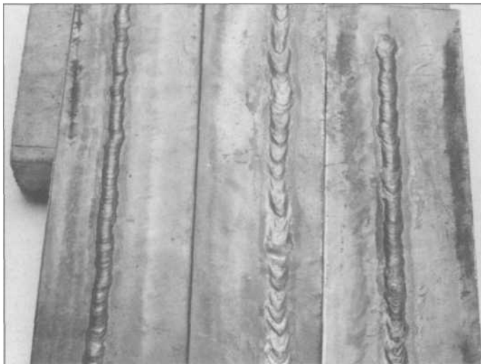
3.25 Heat in gas welding is controlled by matching the gas flow and tip size to the thickness of material. Your welding travel speed and tip-to-work distance will control the puddle size and penetration. With all things right, you should be able to heat your first puddle molten in about six seconds, then move along to make your bead. At left is a bead run too cold (bead stands up), at center is one run too hot and too fast, and at right is a better bead with good width and penetration.
