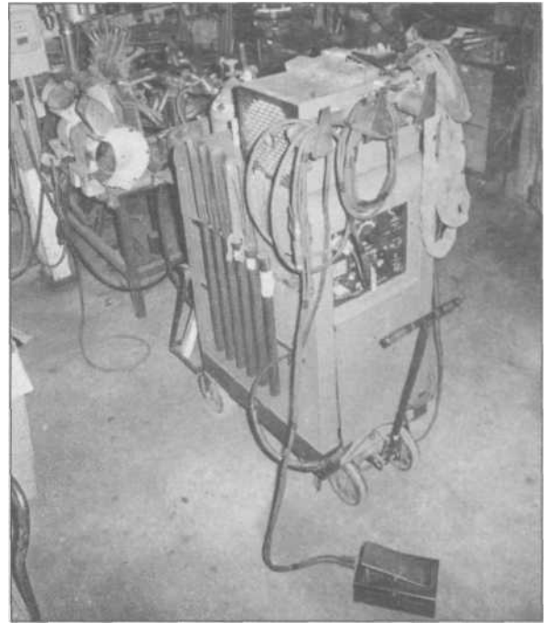
6.20 This is a TIG welder of some years back. Today's current crop of TIGs are half this size. The water-cooling unit here is mounted on top, and at left is a rack of metal tubing holding various welding rods. The foot-pedal amperage control is in front.
