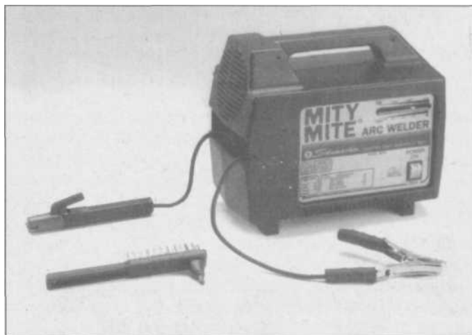
4.30 The Eastwood Company markets a lot of equipment and supplies for auto restoration, and this is their small 110V arc welder. At its maximum of 70 amps, it delivers a 10% duty-cycle, so you won't be welding any bridges together, but it only weighs 26 pounds, so it's extremely portable and welds up to 3/16-inch.
