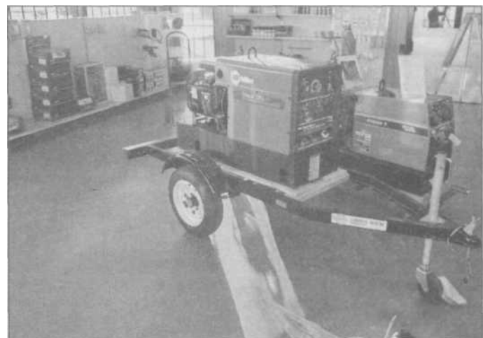
4.9 Contractors often use an engine-driven arc welder mounted on a truck bed or a small trailer. Besides powering the welder, the gas engine also has a large generator to run power tools in a remote work site.
