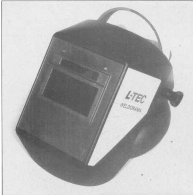
8.4 Another L-TEC helmet, the Weldorama offers a clear sight plate above the welding lens, so the weldor can keep the helmet down, and then just shift his eyes to the dark lens when he is ready to weld.
