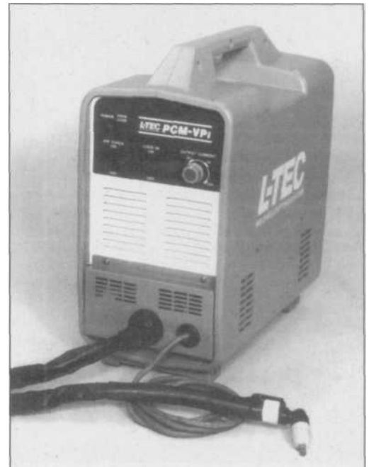
7.8 Another quite-portable plasma machine is the PCM-VPI from L-TEC, which offers cuts up to 5/8-inch in steel, variable amps from 10-40, and a 60% duty-cycle at its rated maximum. It operates on 220V current.
