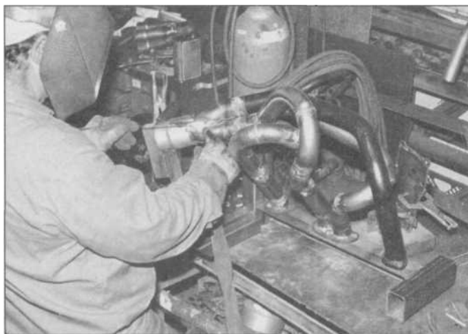
6.5 Where precision welds are involved, especially in tight quarters such as on this stainless-steel race-car header, TIG welding's wide range of operator control is seen as an advantage.
