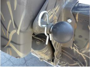
engine facing the boat. While lifting the engine with your left hand, raise the engine upward to line up the tab on the base plate with the engine mount plate. Push the travel lock ball inward to lock the engine upward. Secure the travel lock with the travel lock pin.
