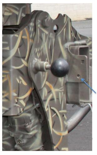
Use silicone to seal the bolt holes. Do not over tighten the bolts and crush the mount or boat transom.
