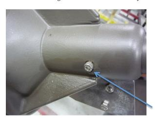
Remove the pressure release bleed screw and grease the drive. Grease until clean grease comes out the bleed screw hole. Replace the bleed screw.
