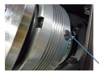
Procedure: Remove one of the fill/drain screws and place it at the 12 o clock position.
