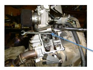
When you feel air coming out (compression stroke) then turn slowly. Look in the spark plug hole with a flashlight and turn the shaft until you see the piston rise to its max point. Turn it just a little bit more till it drops ¼" and then set the valve clearance (this is ¼" past Top Dead Center - TDC).
