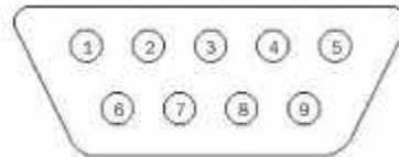
Figure 37 - RS-232 DB-9 pin designations
