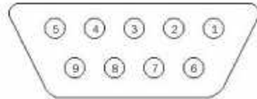
Figure 40 - RS-422/485 DB-9 pin designations
