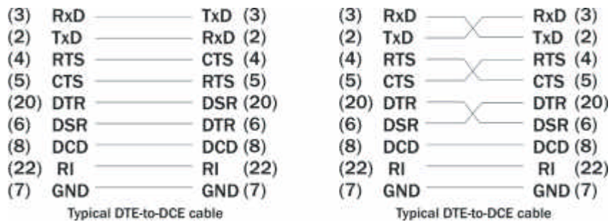
Figure 39 - Cabling requirements for RS-232C devices
