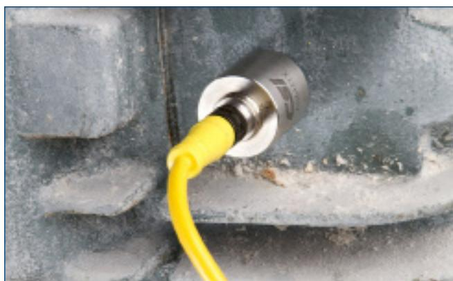
*The triaxial accelerometer allows for the collection of vertical, horizontal and axial data from the same location simultaneously.*
