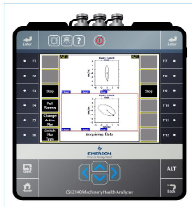
Monitor dual orbit plots from two sleeve bearings on the turbine, fan, or other critical machinery to determine if the startup can continue.
