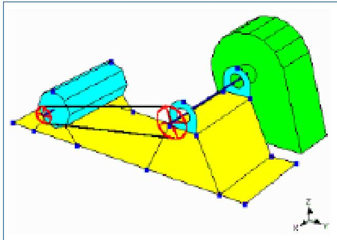
*View wireframe animations in ODS software to identify structural problems with the machine during operation.*
