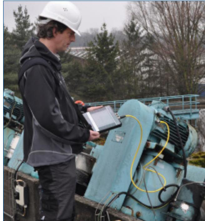
*The CSI 2140 Machinery Health Analyzer makes data collection and advanced analysis easier and more efficient.*
