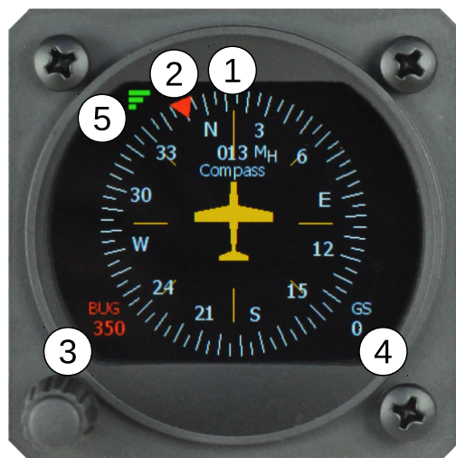
Figure 7: Horis Direction Indicator screen with the markings.
