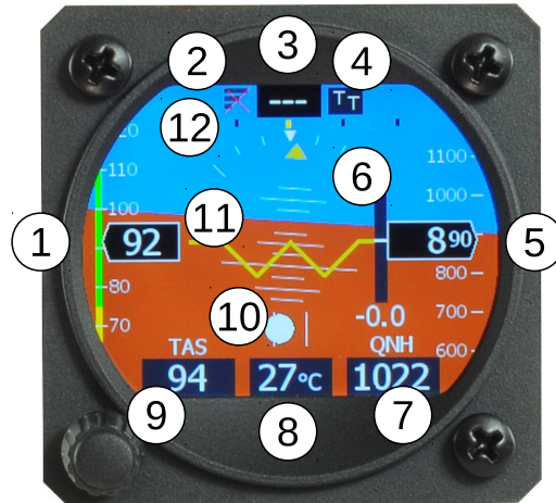
Figure 6: Horis AD-AHRS screen with the markings.
