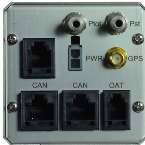
Figure 3: Back view of the instrument with connections. 57 mm version is shown.
