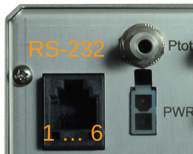
Figure 4: Illustration of the pin out of the RS-232 port.
