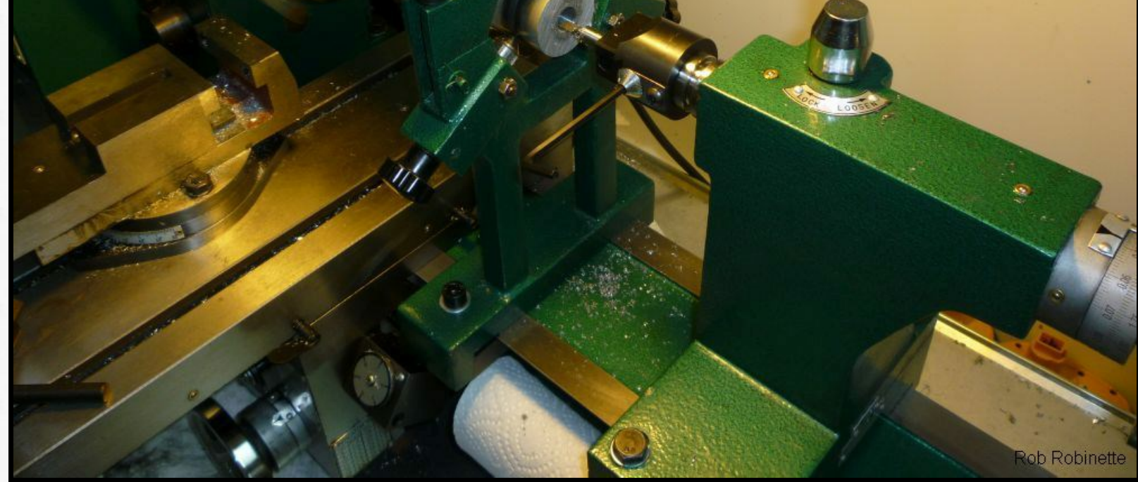
Boring the tap hole to the pre-tap size. This is not necessary if you have the correct size drill bit as listed above.
