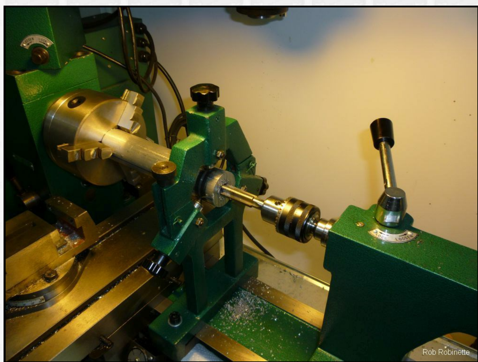
Tapping the baffle--Do not try to use lathe power to do this. I used the tailstock to simply hold the tap for perfect alignment with the bullet path. I pushed inward on the tailstock and turned the lathe chuck by hand to start the tap. I did the last half of the tap using a standard tap hand wrench so I could feel when the tap bottomed out. I used a 5/8x24 threads per inch (tpi) tap to match the thread on my 300 Blackout barrel.
