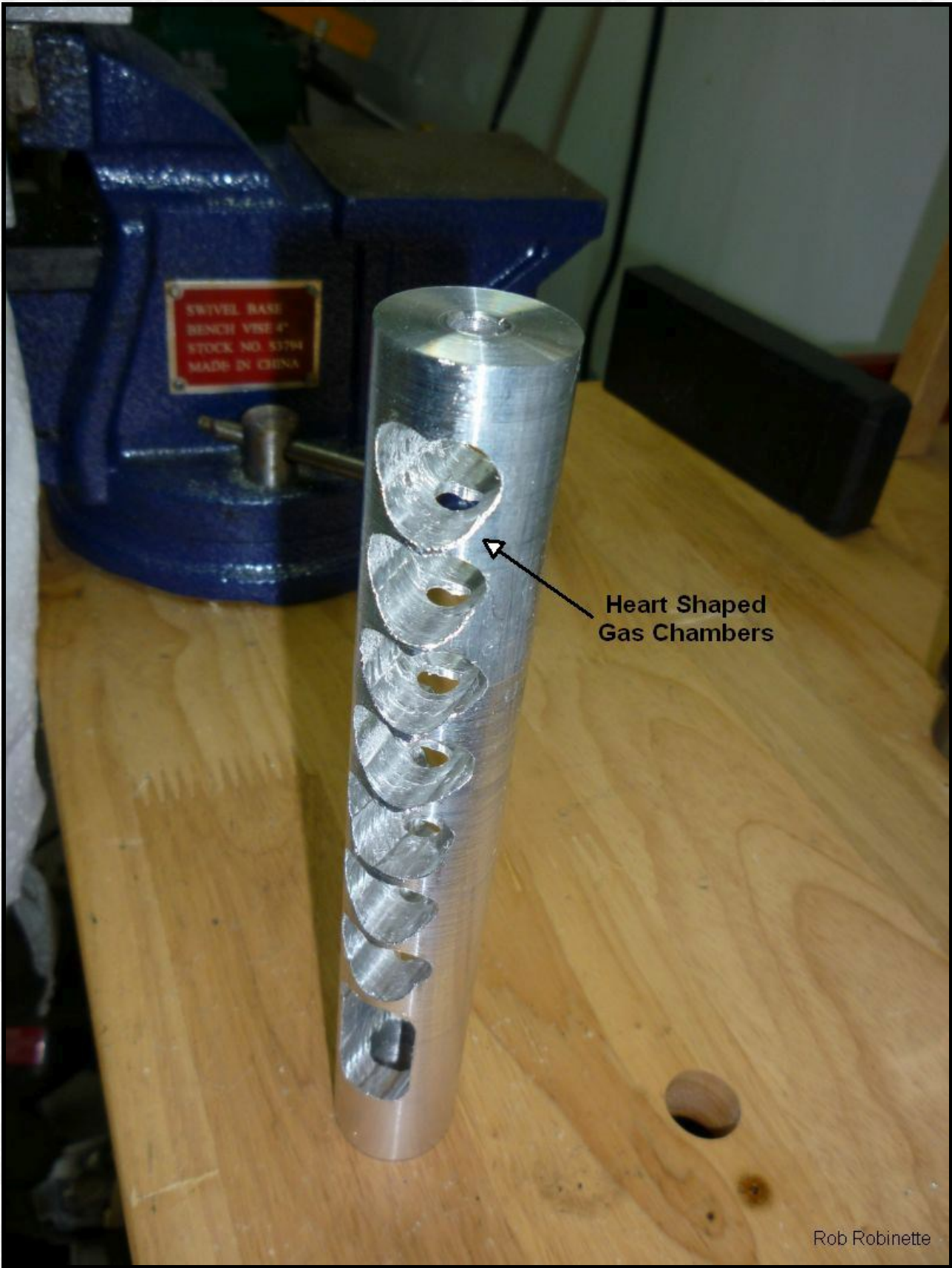
A .22 baffle made of 1 inch solid round aluminum bar. Note the large square blast baffle at the
