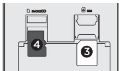
4. Insert a microSD card into the storage card slot with its gold contacts facing down.
