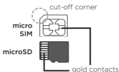
3. Insert the micro SIM card into the micro SIM slot, with the card's gold contacts facing down and cut-off corner facing in.
