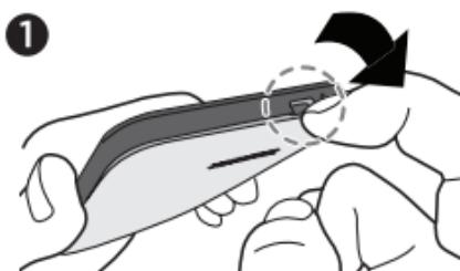
1. With the phone facing away from you, open the back cover from the notch at the bottom (where the charger connector is located).
