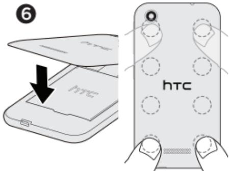
6. To place the back cover, align the phone onto the top part of the back cover first. Then press the sides and the lower part down from top to bottom to lock the cover into place.
