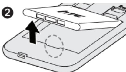
2. Before inserting the micro SIM and microSD™ cards into the slots, you need to remove the battery.
