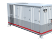
FusionModule1000A20 20 ft stand-alone with 4 racks Total IT Power: \leq 24 kW Power Density: \leq 6 kW/Rack
