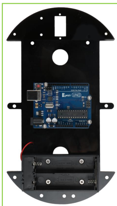
Figure 3.1.26 Effect diagram of battery box installation
