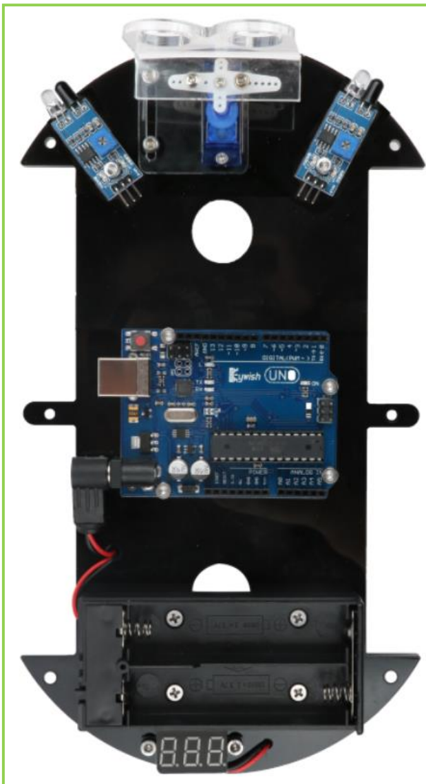
Figure 3.1.36 Effect diagram of voltage display module and DC head installation
