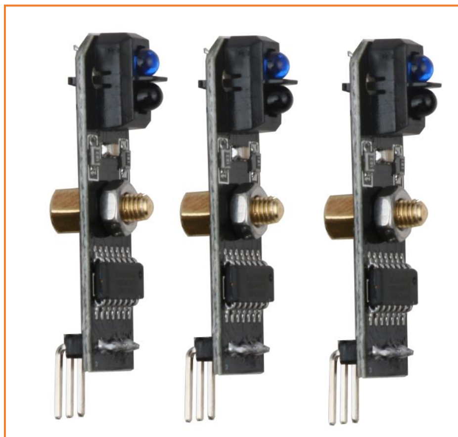
Figure 3.1.16 Effect diagram of copper column of tracking moduble installation
