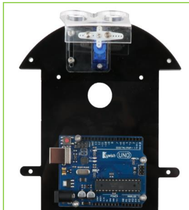
Figure 3.1.30 Effect diagram of rudder wing and ultrasonic bracket installation
