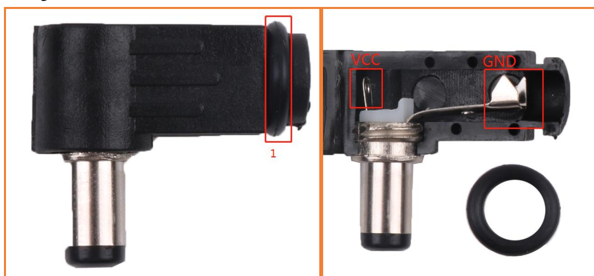
Figure 3.1.30 Schematic diagram of solder DC power supply head
