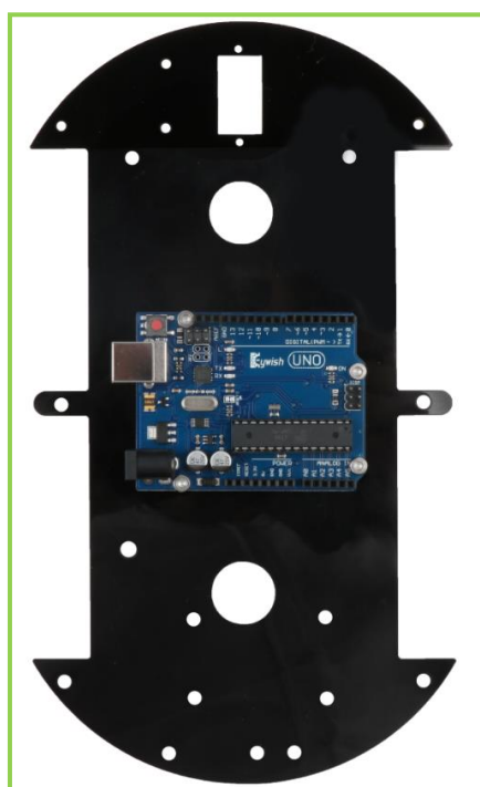
Figure 3.1.20 Effect diagram of Keywish Uno R3 board installation
