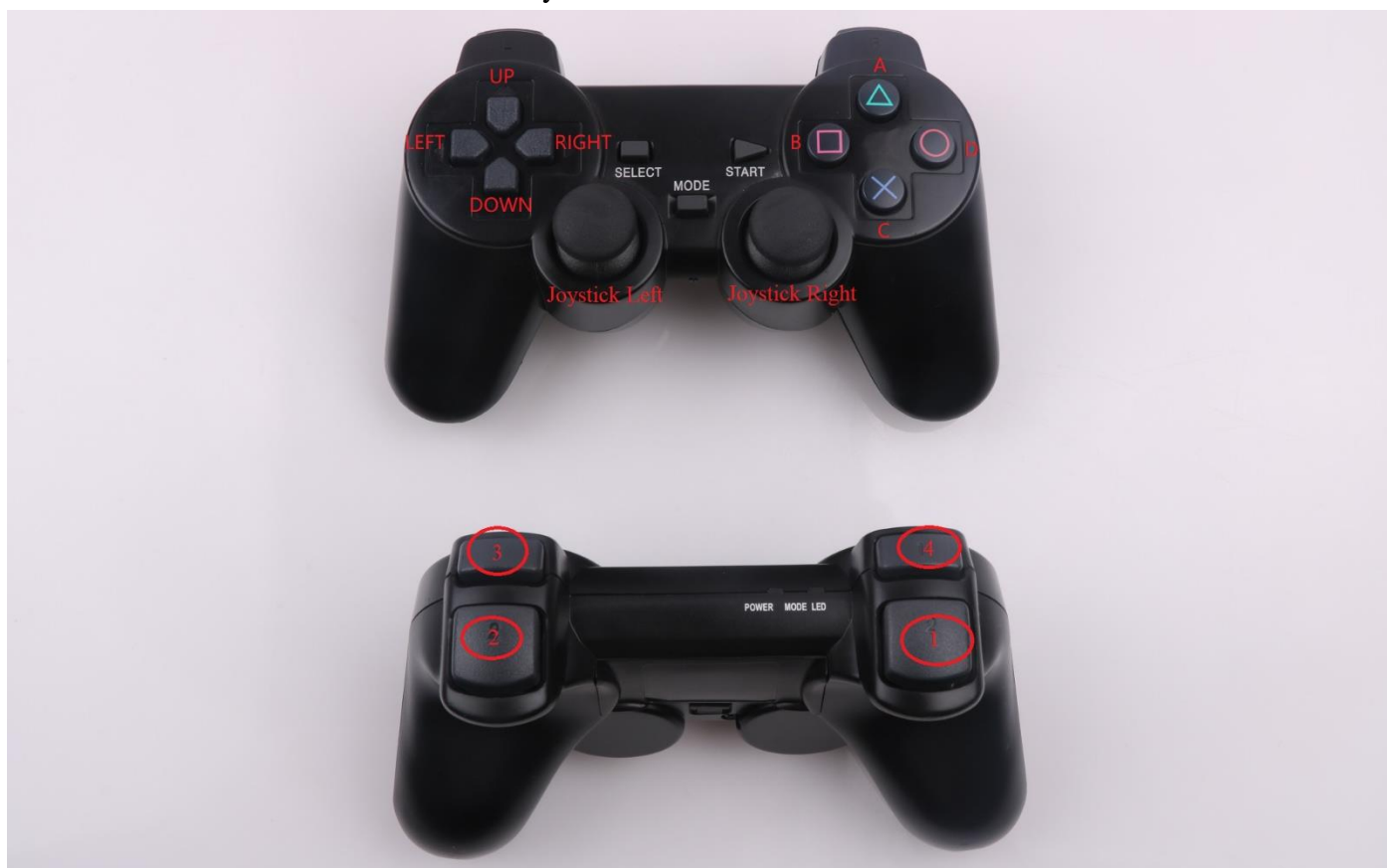
Figure .3.2.60 Functions of PS2 Handle Buttons
