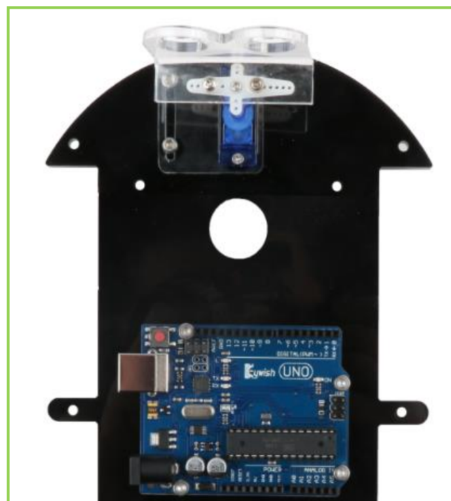
Figure 3.1.26 Effect diagram of rudder wing and ultrasonic bracket installation
