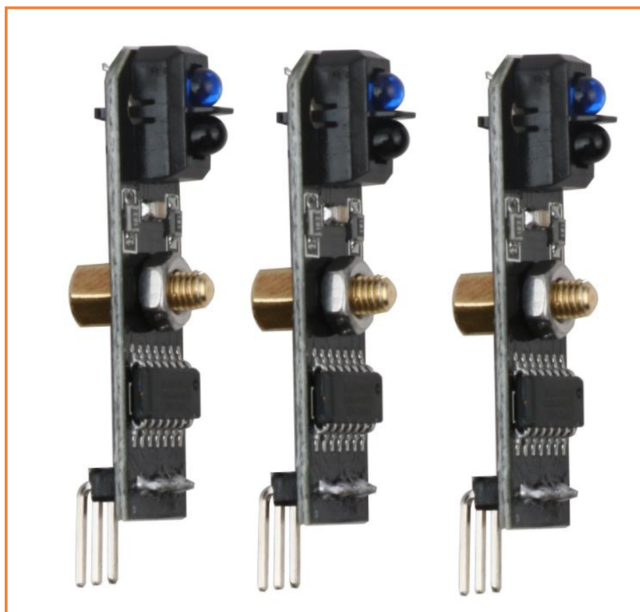
Figure 3.1.12 Effect diagram of copper column of tracking module installation
