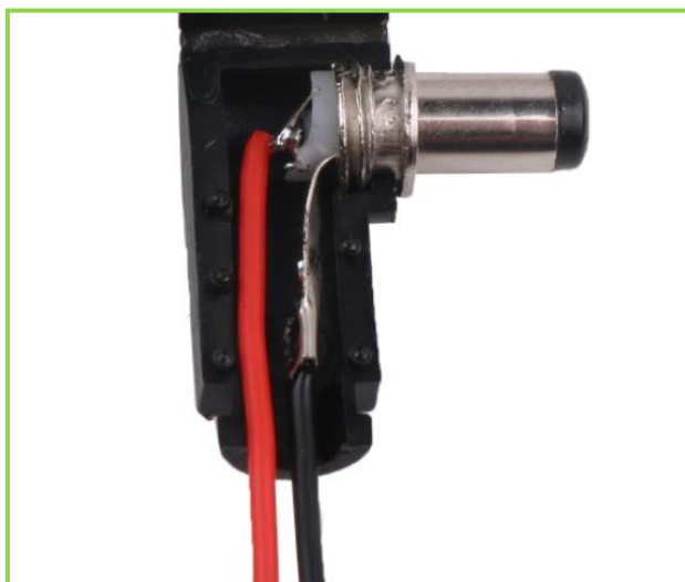
Figure 3.1.31 Effect diagram of solder DC power supply head
