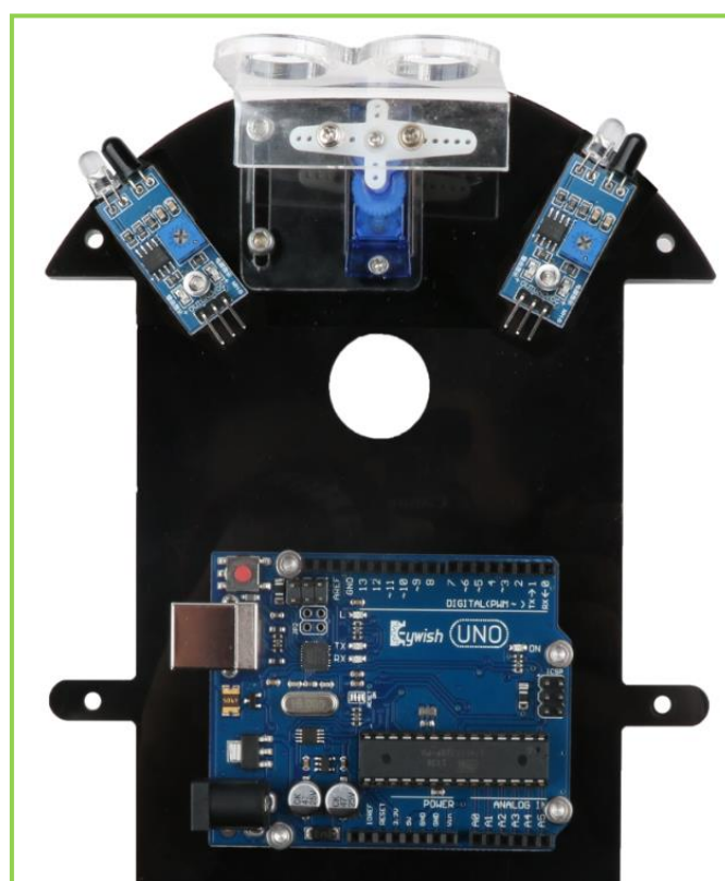
Figure 3.1.28 Effect diagram of infrared obstacle module installation
