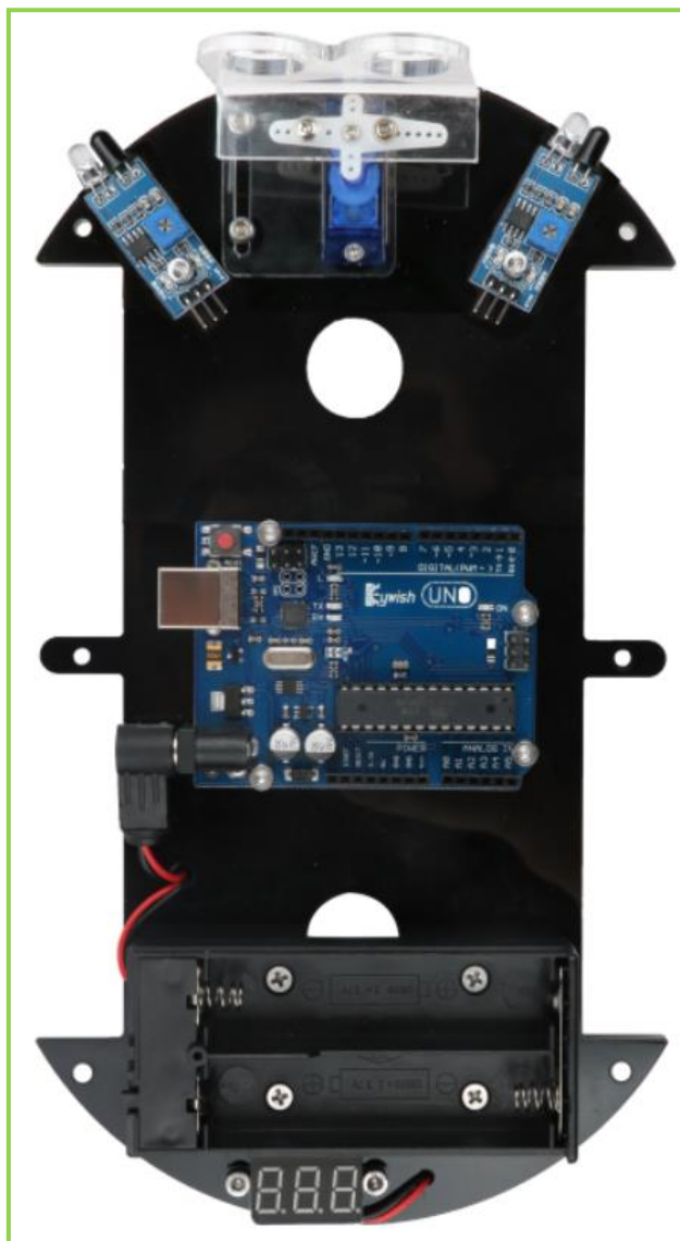
Figure 3.1.32 Effect diagram of voltage display module and DC head installation
