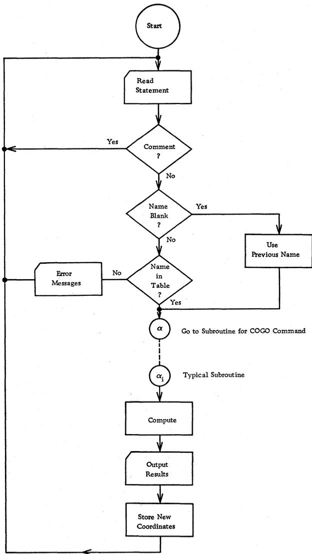
FIGURE 3. Simplified flow diagram of COGO
