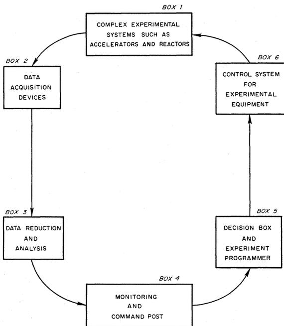
FIGURE 1. General schematic of integrated data analysis and control system for complex experiments
