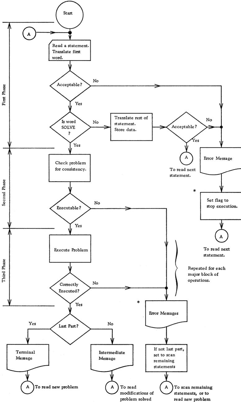
FIGURE 4. Simplified flow diagram of STRESS
