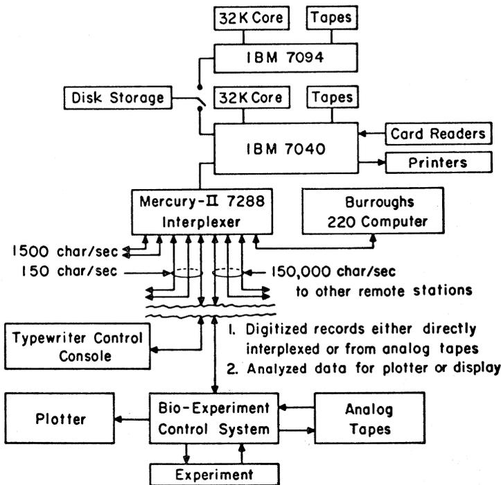
FIGURE 3. Schematic diagram of computer layout for research in visual perception
