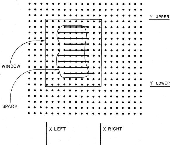
FIGURE 8. Line segments and cells generated by CELL CONSTRUCTION ALGORITHM
