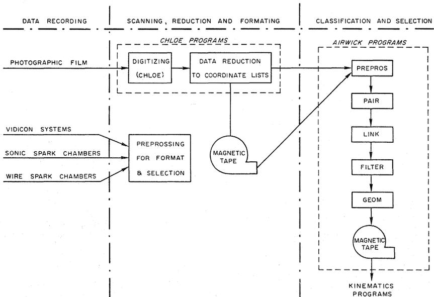
FIGURE 4. Schematic of the flow of data in the Argonne system
