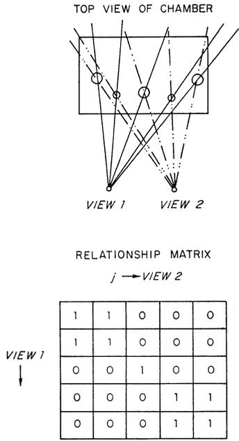
FIGURE 9. Schematic of top of spark chamber with five sparks and corresponding relationship matrix
