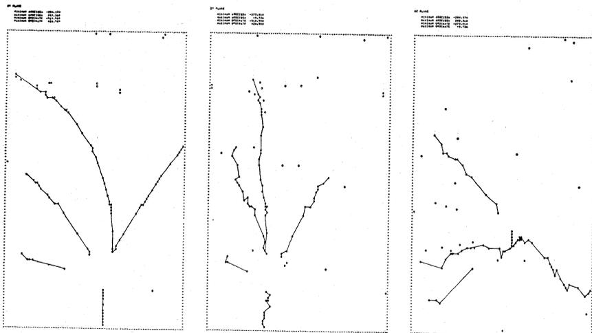
(6b) The event after processing by AIRWICK, showing the reconstructed tracks. Random sparks not on the tracks have now been eliminated.
