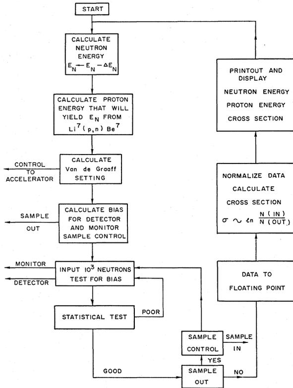
FIGURE 3. Schematic flow chart of first program run on the system depicted by Figure 2
