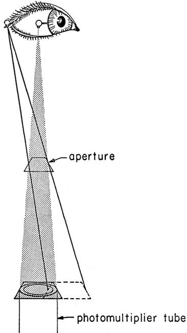
FIGURE 10. Contact lens and photomultiplier used for recording horizontal component of eye movements
