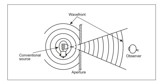
Figure 1-7. Divergence of conventional light beam
