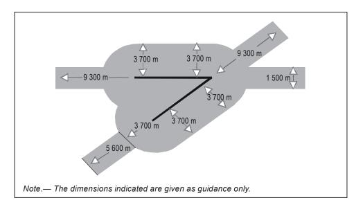
Figure 5-2. Multiple runway laser-beam free flight zone (LFFZ)
