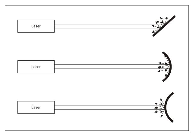
Figure 1-12. Diffuse reflectors
