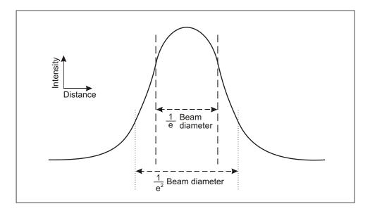
Figure 1-5. Beam diameter
