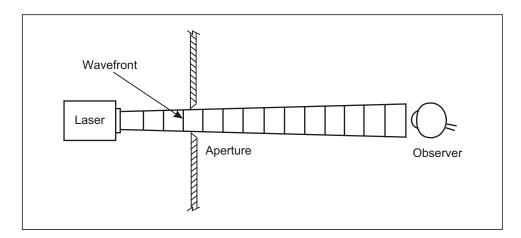
Figure 1-8. Divergence of laser beam
