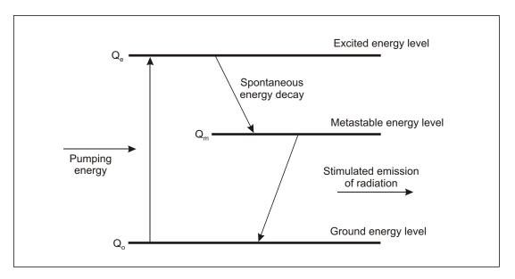
Figure 1-3. Diagram of three-level laser energy
