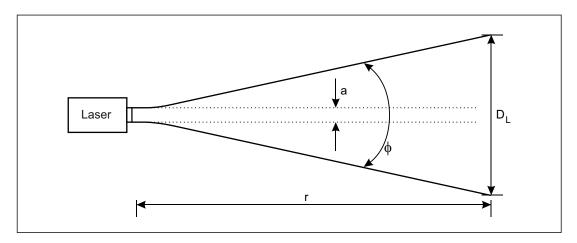
Figure 1-9. Geometry of laser beam
