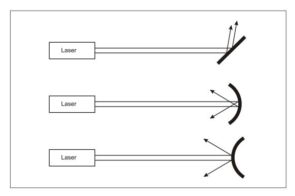
Figure 1-11. Specular reflectors
