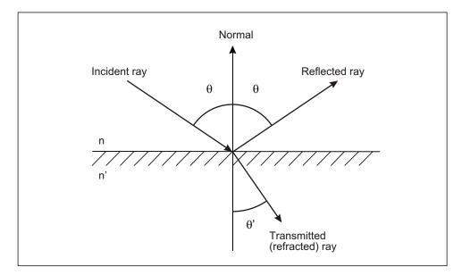
Figure 1-10. Light ray incident to a glass surface
