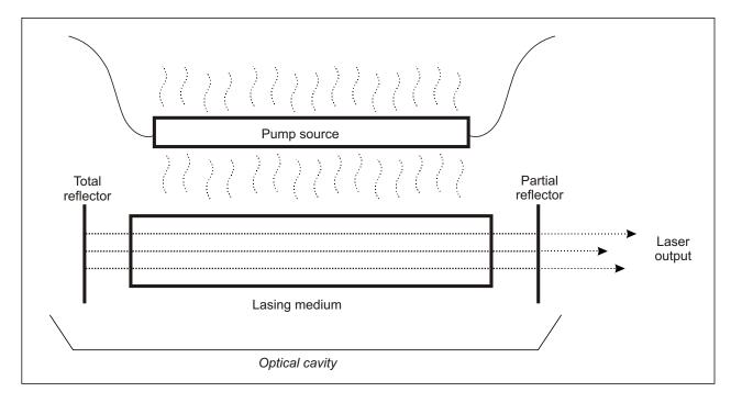
Figure 1-2. Diagram of solid state laser
