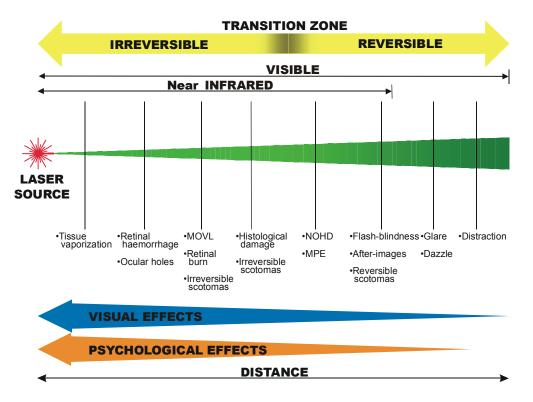
Figure 3-3. Ranges of laser beam bioeffects
