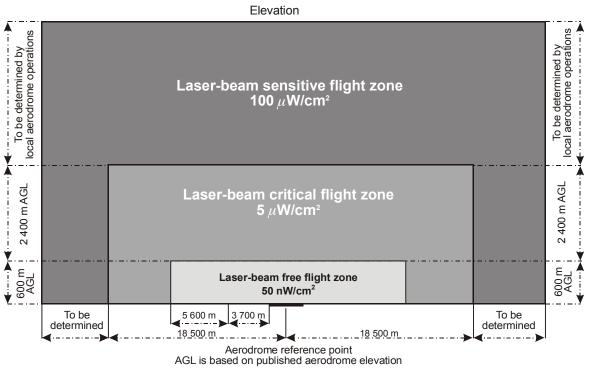
Figure 5-3. Protected flight zones with indication of maximum irradiance levels for visible laser beams
