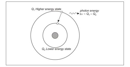
Figure 1-1. Emission of radiation from an atom by transition of an electron from a higher energy state to a lower energy state
