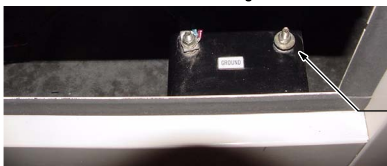
Figure 3-4 Frame Ground Connection
