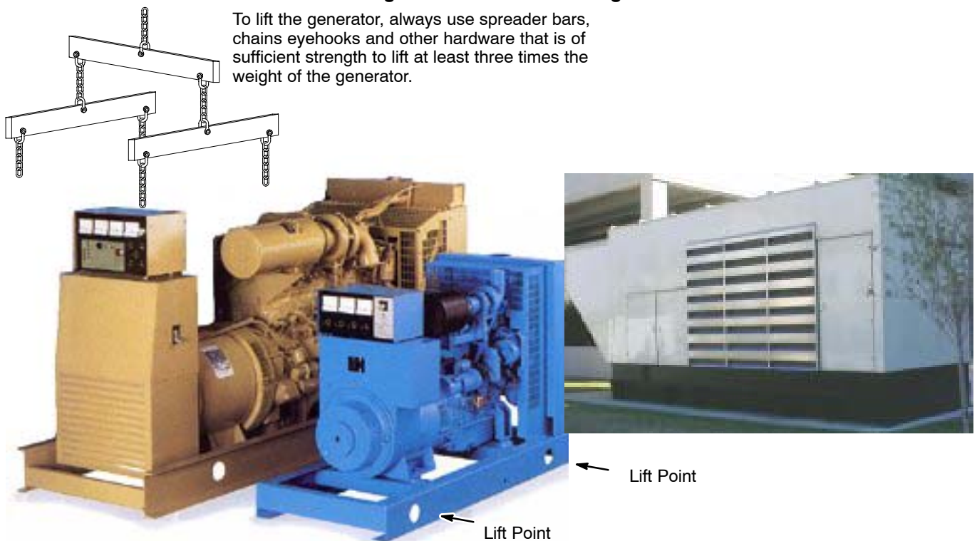
Figure 3-1 Generator Lifting
