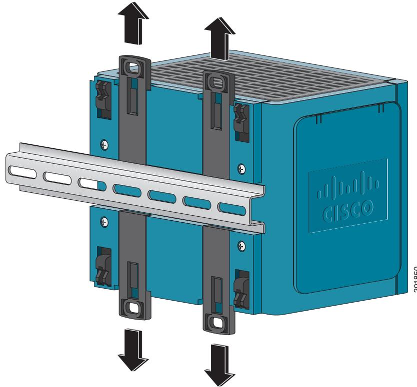
**Step 4** Remove the switch from the DIN rail.
