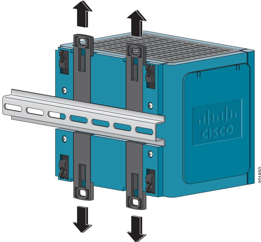
**Step 4** Remove the switch from the DIN rail.
