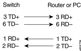
**Figure C-6 Two Twisted-Pair Crossover Cable Schematic**
