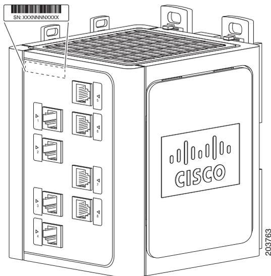
**Figure 3-3** Serial Number Location for the Cisco PWR-IE3000-AC Power Converter
