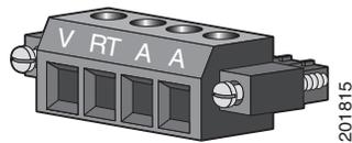
**Step 2** Identify the positive and return DC power connections on the connector. The positive DC power connection is labeled V, and the return is the adjacent connection labeled RT. See [Figure B-12](#).
