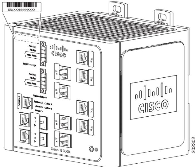
**Figure 3-2** Serial Number Location for the Cisco IEM-3000-8TM and the Cisco IEM-3000-8FM Module
