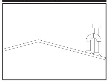
FIG. 21 Air Inlet Cap for Rooftop Termination
