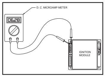
FIG. 65 Flame Current Measurement on the HSI Module
