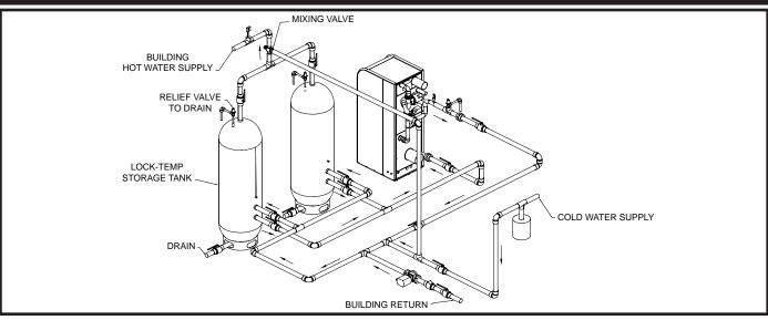
FIG. 84 Single Water Heater Piping with Two Storage Tanks
