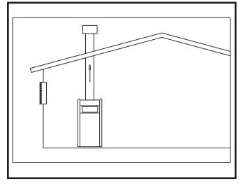
FIG. 8 Combustion Air from Outside - Single Opening
