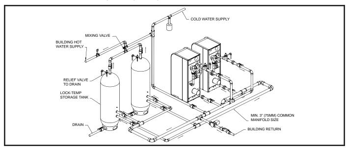
FIG. 86 Multiple Water Heater Piping with Multiple Storage Tanks
