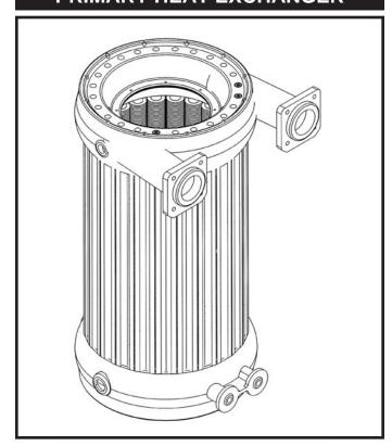
FIG. 38 Primary Heat Exchanger
