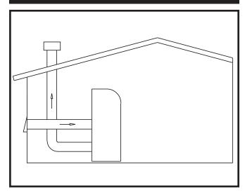
FIG. 27 Vertical Intelli-Vent Installation – Sidewall Combustion Air Inlet
