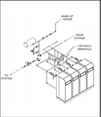
FIG. 81 Primary/Secondary Piping of Multiple Boilers
