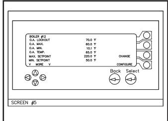
FIG. 56b Command Display Data Screen
