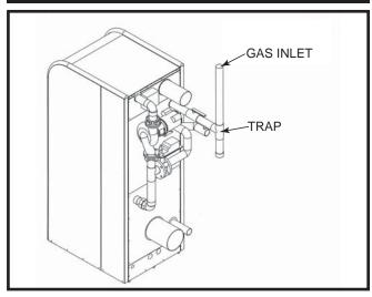
FIG. 34 Gas Line Connection to Unit with Sediment Trap and Manual Main Gas Shut-off Valve
