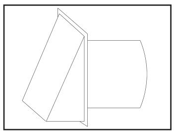
FIG. 25 Air Inlet Cap for Sidewall Termination
