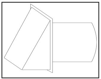
FIG. 33 Air Inlet Cap for Sidewall Termination
