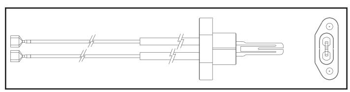
FIG. 64 Hot Surface Igniter
