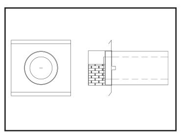
FIG. 24 Sidewall Vent Cap
