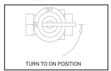
FIG. 75 Gas Cock with Handle in "ON" position
