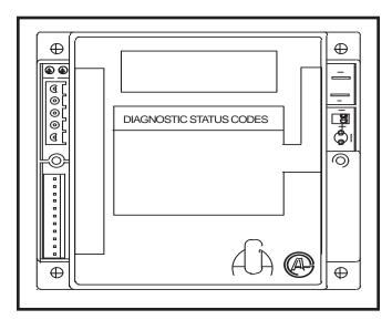
FIG. 63 Hot Surface Ignition Control Module
