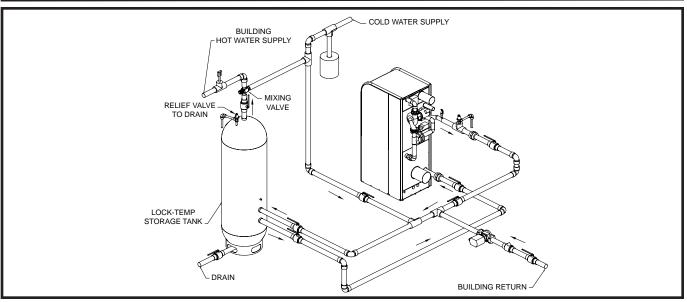
FIG. 83 Typical Water Heater Piping with Storage Tank
