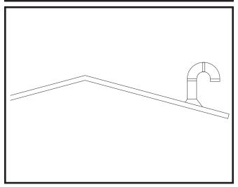
FIG. 30 Air Inlet Cap for Rooftop Termination
