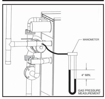
FIG. 35 Gas Supply Pressure Measurement
