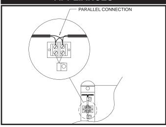
FIG. 59 E-Bus Connection to Controls
