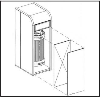
FIG. 77 Location of Primary Heat Exchanger
