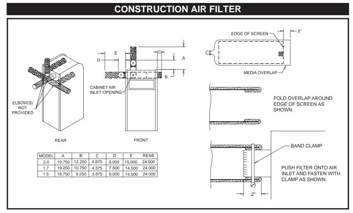
FIG. 9 Construction Air Filter
