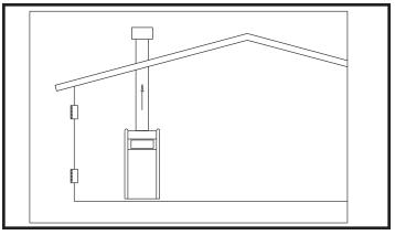
FIG. 5 Combustion Air Direct from Outside
