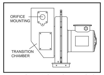
FIG. 69 Combustion Air Blower and Transition Chamber
