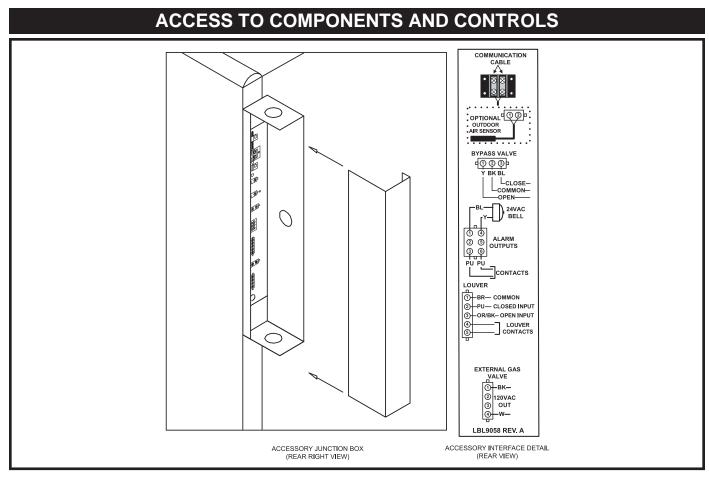
FIG. 46 Component and Auxiliary Controls Connections with Junction Box
