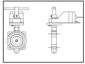
FIG. 41 Bypass Valve and Actuator Assembly
