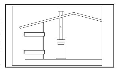
FIG. 6 Combustion Air Through Ducts
