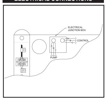
FIG. 45 Electric Power Connections - Controls and Pumps
