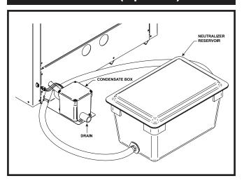
FIG. 71 Location and Connection of Neutralization Reservoir
