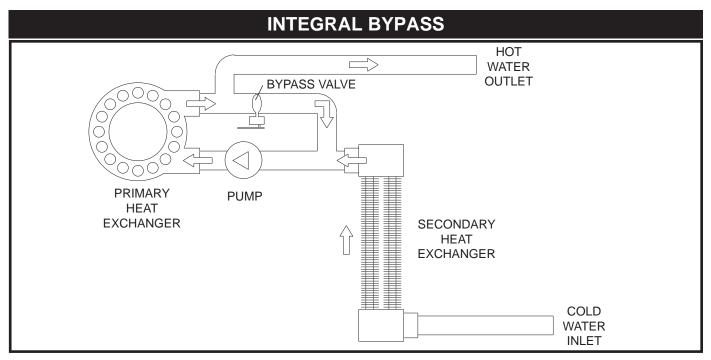
FIG. 40 Bypass Piping with Valve Actuator and Pump
