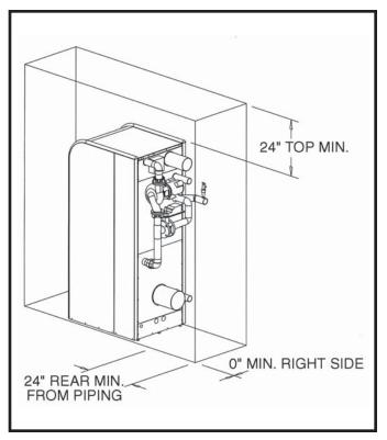
FIG. 4 Recommended Service Clearances - Rear
