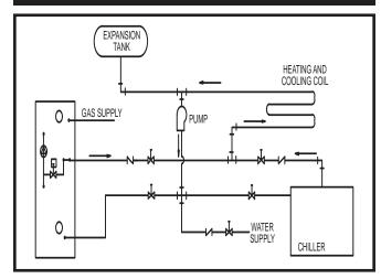
FIG. 82 Installation with a Chilled Water System
