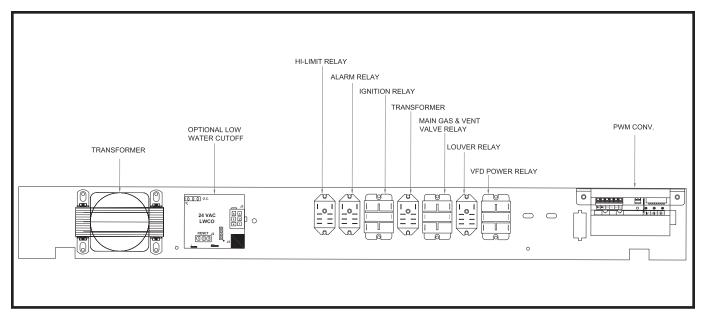
FIG. 48 Transformer and Relay Locations
