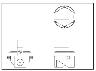
FIG. 44 Diaphragm Gas Valve
