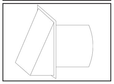
FIG. 28 Air Inlet Cap for Sidewall Termination
