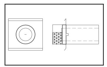
FIG. 32 Sidewall Vent Cap
