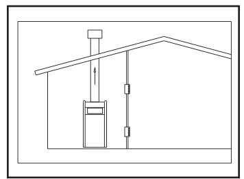
FIG. 7 Combustion Air from Interior Space
