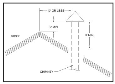
FIG. 13 Vent Termination from Peaked Roof - 10 Feet or Less from Ridge
