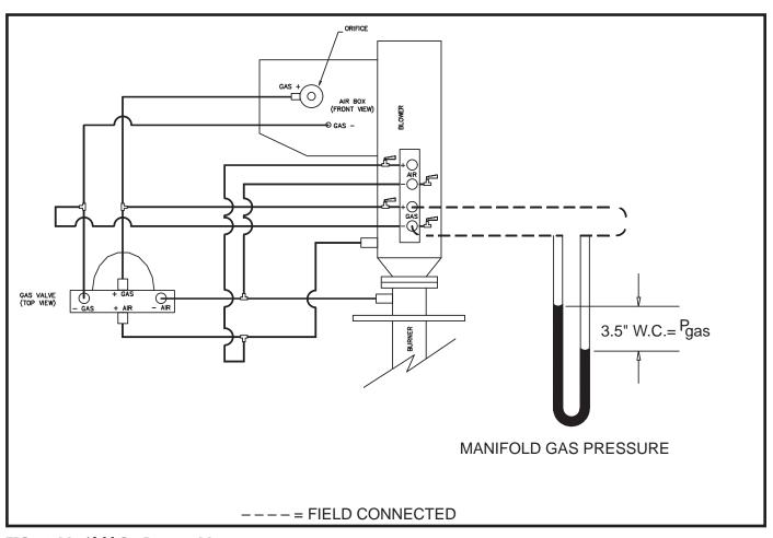
FIG. 36 Manifold Gas Pressure Measurement
