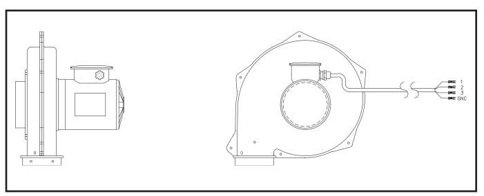
FIG. 68 Combustion Air Blower
