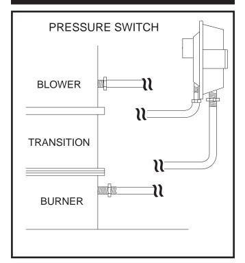
FIG. 51 Low Air Pressure Switch
