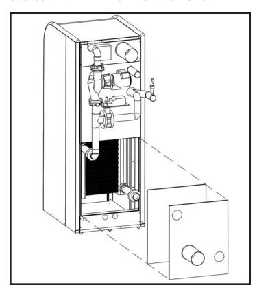
FIG. 78 Location of Secondary Heat Exchanger
