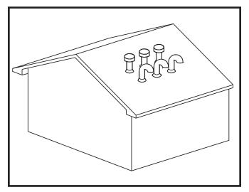
FIG. 22 Multiple Vertical Direct Vent Installations
