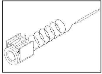
FIG. 62 High Water Temperature Control
