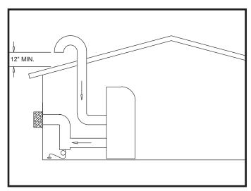
FIG. 29 Horizontal Intelli-Vent Installation - Rooftop Combustion Air Inlet
