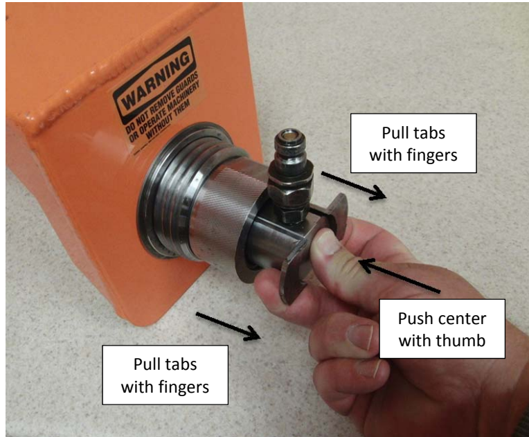
Picture 11B - Activation of the safety interlock
