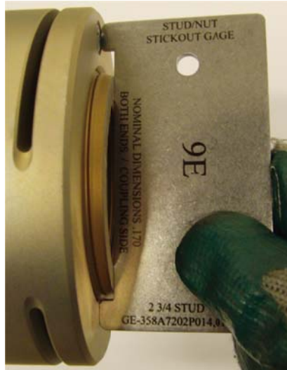
Picture 6C – Use of Stick-Out Gage
