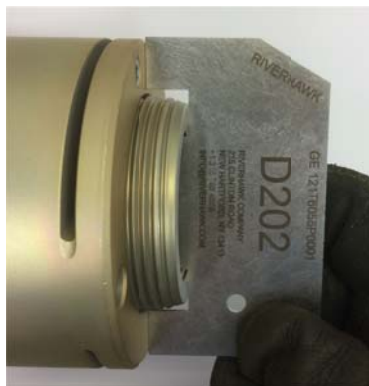
Picture 6B – Use of Stick-Out Gage on the D602 HPIP-LP Flange Joint Note: The D202 stick-out gage is used on this special application
