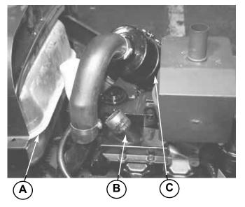
A. FLEXIBLE HOSE B. HEAT COLLECTOR SHIELD C. AIR FILTER
