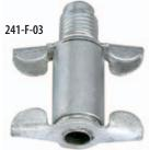
Pinch-off tube on hermetic compressor is cut off and 241-F is placed on tube. Charging line is connected to flare end of 241-F.
