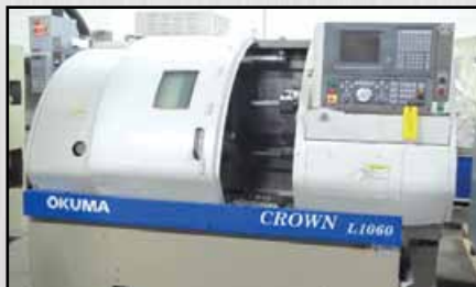
1999 Okuma Crown L1060 Model 762S-SB OPS-700L Control, Travel 20x8" 22" swing 4200RPM
