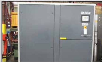
Atlas Copco Ga75FF 100HP Air Compressor - Bui It in AIR DRYER - 433 CFM
