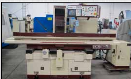
Chevalier FSG-1640TXII - Hydraulic Automated Surface Grinder - 16 x 40" magnetic chuck
