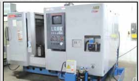
1998 MAZAK HTC 400 CNC horizontal machining center MAZA- TROL MPLUS 16" DUAL pallets travels 22x20x20" 10000 RPM
