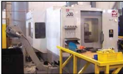
2007 Haas EC-500 CNC Horizontal Machining Center - Haas Controller - TRAVELS X-Axis 32" Y-Axis 20" Z-Axis 28"
