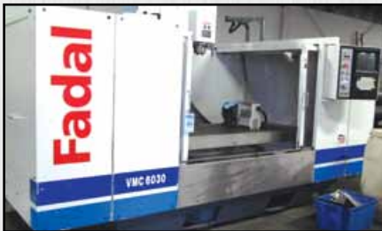
2 X FADAL VMC 6030 CNC VERTICAL MACHINING CENTER travel 60x30x28" 10000RPM with 4th Axis
