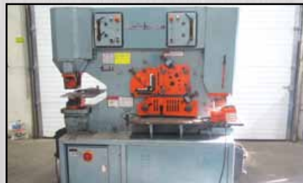
Scotchman 85 Ton Ironworker model D.O. 8514-20M - 230V 3 phase - 14" deep throat with foot pedal
