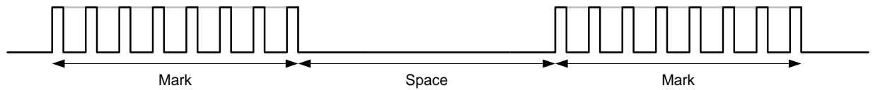
Figure 31. IR Coded message with carrier
