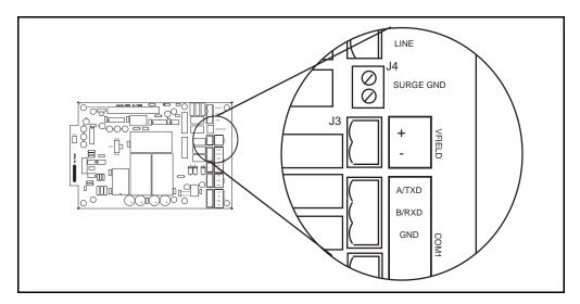
Figure 2-5: Field Power Terminal Block
