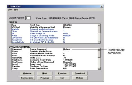
Figure 5-1: Varec 6000 Servo Gauge (STG) Tank Point edit dialog box
