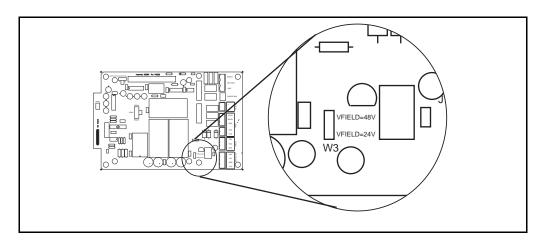
Figure 2-8: Selection Jumper W3
