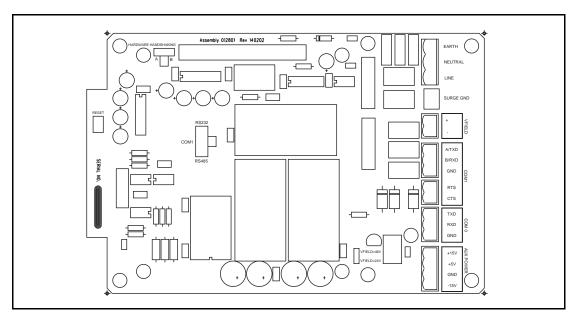
Figure 2-2: The Tank Gate Interface Motherboard
