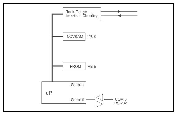
Figure 2-3: Tank Gate Interface Functional Block Diagram
