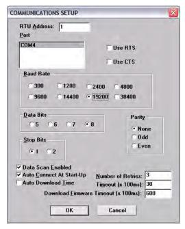
Figure 8-16:Port Communications Setup dialog
