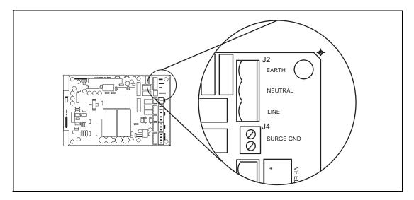
Figure 2-4: AC Input Terminal Block
