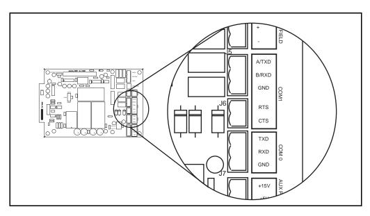
Figure 2-10: COM1 J5 Terminal Block
