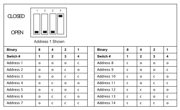
Figure 3–2: ID DIP Switch settings
