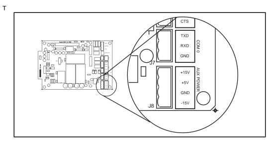
Figure 2-6: DC Input Voltage Terminal Block
