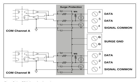
Figure 3-4: COM channels schematic
