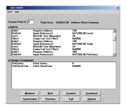
Figure 4-3: Configure the GWBLK in View RTU
