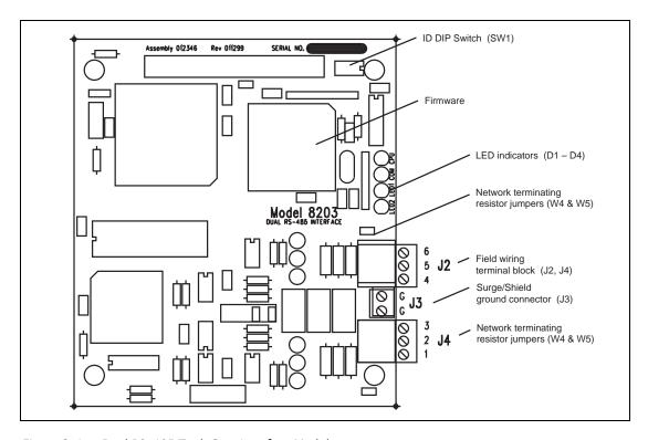
Figure 3-1: Dual RS-485 Tank Gate Interface Module
