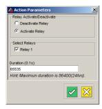
We recommend that you create a second relay Action to deactivate the first one. The second Action will deactivate the Relay and disable the Inhibit Scanner function.
