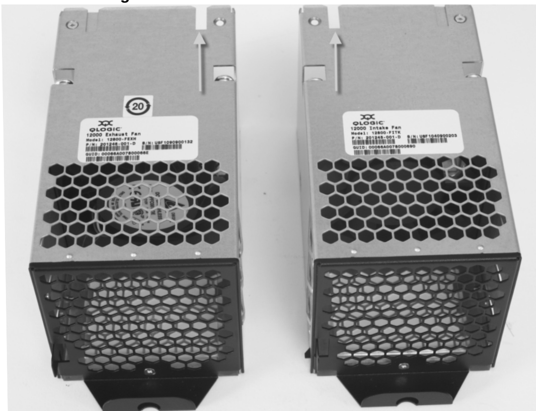
Figure D-3 .12800 Intake and Exhaust Fans
