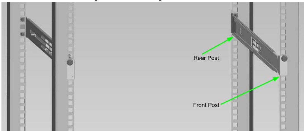
Figure 1-8 Installing the Rack Rails
