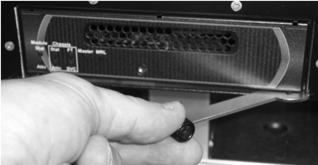
Figure D-8 .12800 Management Module Removal
