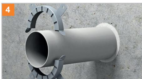
A suitable fire protection collar must be utilised. For pipe penetrations through floors, there must be a fire protection collar arranged to the bottom side of the floor. For pipe penetration through walls, there must be a fire protection collar arranged on each side of the wall.
