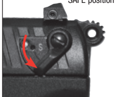
fig. 1 Manual safety in SAFE position
