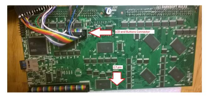
If you have a revision 5 or above, you'd be ok with a PAL G or a PAL F+Cable. If you already have a PAL F, you have to lift pin 7 of PAL 3 so that doesn't go into the socket and doesn't make contact and solder a jumper wire into the pin J17 that I explained for revision 3 and 4.
