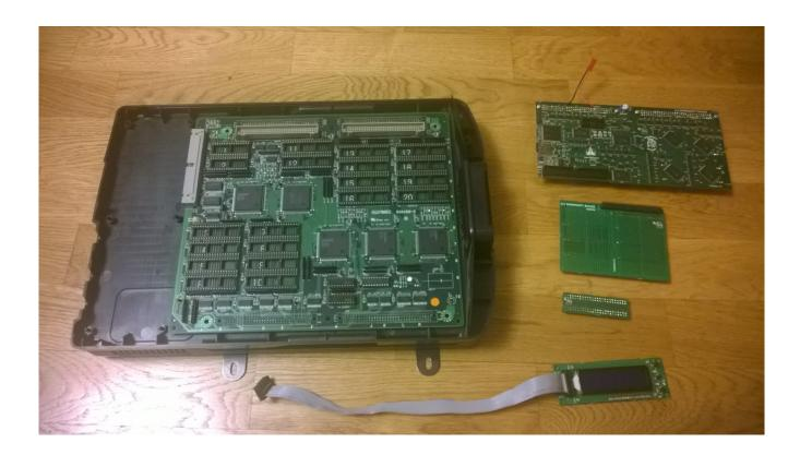
First, proceed to install the smaller PCB. Check that the PCB is placed as in the picture below. First just lay it, to make sure all the pins are in the right place.
