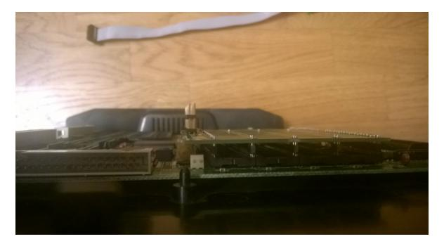
Now you can proceed to installing the big PCB. First make sure that it has arrived undamaged to you. It is important that no pins have been bent. Notice that only the top of the pin should go inside. This is the part marked in red.
