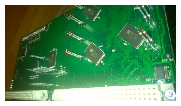
The first thing is to align the white connectors with the ones in the B Board like you can see below. Again you need to carefully look at the pins while you insert them in the Eprom socket to make sure that everything is aligned and the pins insert in the right place.
