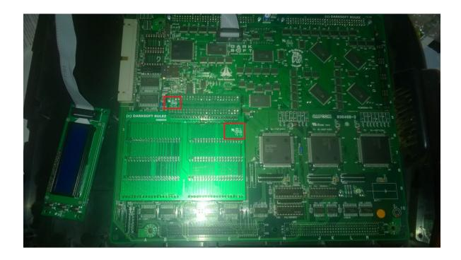
Your kit also includes an LCD screen module with 3 buttons to choose which game to load. The buttons and the cable are connected to the bigger PCB's 14-pin socket and you can take that cable outside the B Board case through the register opening in one of the sides. You will be able to change games with the lid closed.
