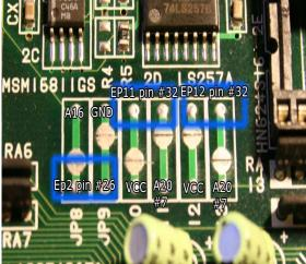
You can try with a tester in continuity mode (makes beep if two points are electrically connected). If you hear a beep, then it's Short.
