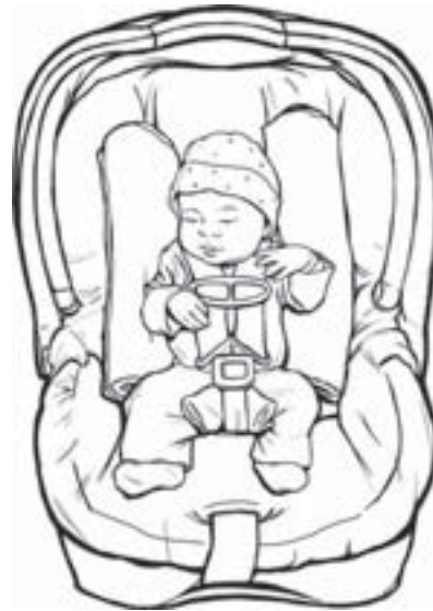
FIGURE 1 Car safety seat with a small cloth between crotch strap and infant, retainer clip positioned at the midpoint of the infant's chest, and blanket rolls on both sides of the infant.
