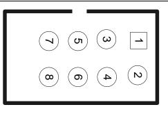
Figure 7. Dual Port USB Header (Top View)
