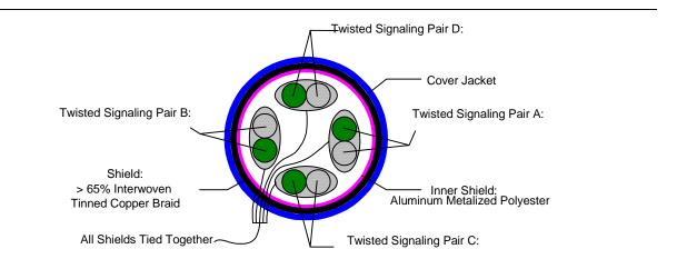
Figure 12. Front Panel Audio Cable Cross-Section
