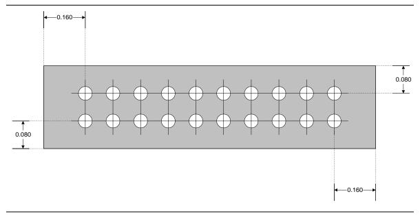
Figure 40. LPC Debug Connector Keep-Out Zone
