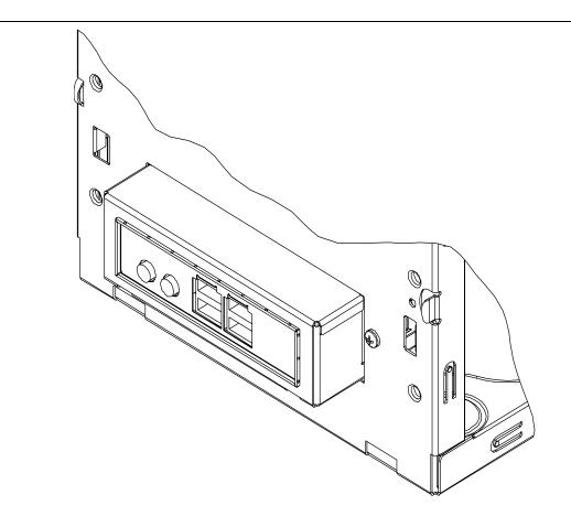
Figure 32. Front Panel I/O Housing and Shield Assembly Reference Design
