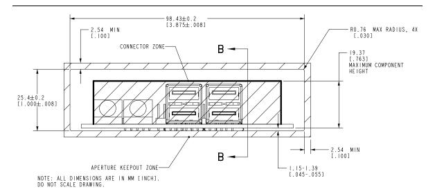
Figure 27. Front Panel I/O Aperture and Interface Board Placement Recommendations
