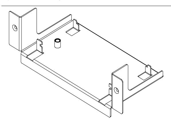
Figure 33. Front Panel I/O Interface Board Support Structure Reference Design
