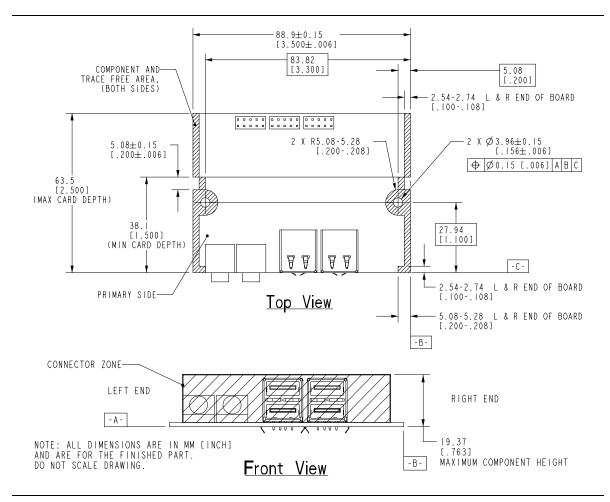
Figure 25. Front Panel I/O Board Dimensions (Top and Front Views)
