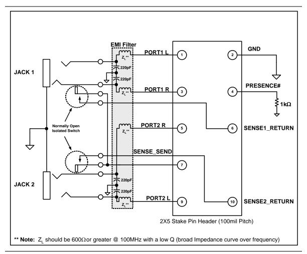
Figure 6. Intel<sup>®</sup> HD Audio Front Panel Dongle Implementation
