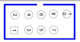
Figure 9. Front Panel IEEE-1394A/B Connector (Top View)
