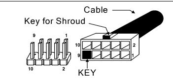
Figure 22. IEEE 1394A/B Cable Diagram
