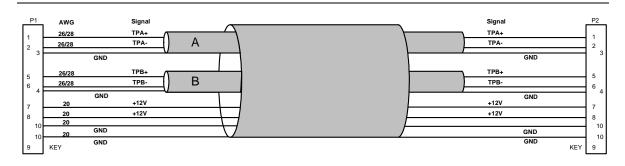
Figure 21. IEEE 1394A/B Cable Wiring Diagram
