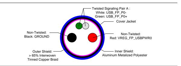
Figure 17. Single Port USB Cable Cross Section
