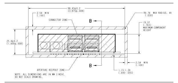
Figure 23. Front Panel I/O Aperture and Interface Board Placement Recommendations
