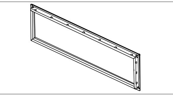
Figure 29. Front Panel I/O Shield Reference Design
