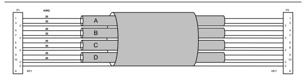
Figure 13. Audio Cable Wiring Diagram
