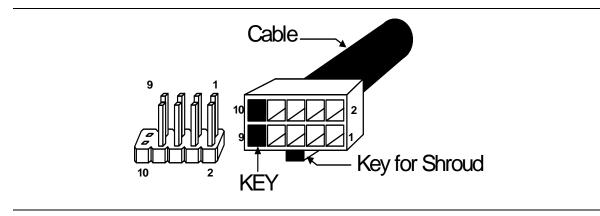
Figure 16. Dual USB Cable Diagram
