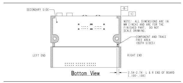
Figure 26. Front Panel I/O Board Dimensions (Bottom View)
