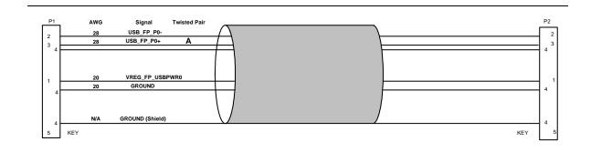
Figure 18. Single Port USB Cable Wiring Diagram
