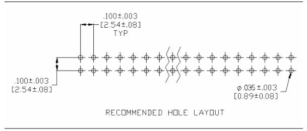
Figure 39. LPC Debug Connector Hole Layout
