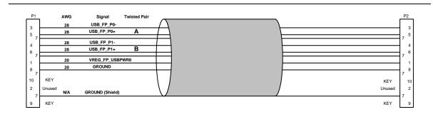
Figure 15. Dual Port USB Cable Wiring Diagram
