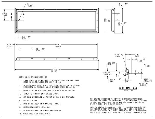
Figure 30. I/O Shield Reference Design
