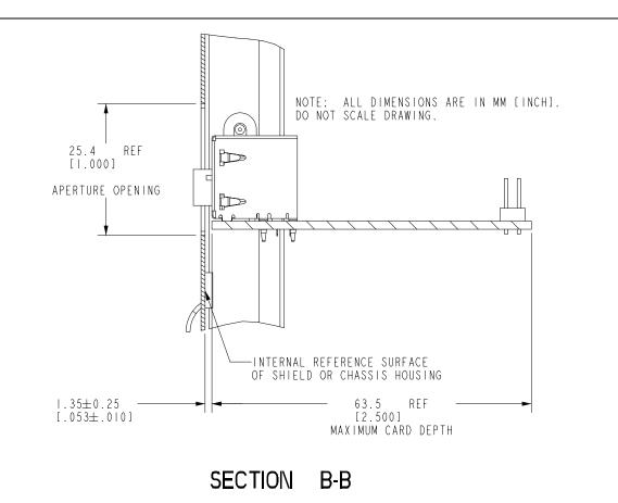
Figure 24. Front Panel I/O Interface Board Placement Recommendations
