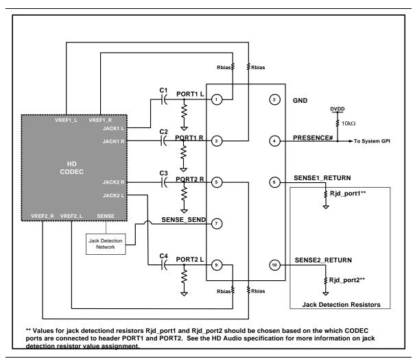
Figure 5. Intel<sup>®</sup> HD Audio Front Panel Analog Header Motherboard Schematic
