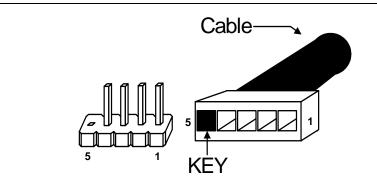
Figure 19. Dual USB Cable Diagram
