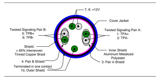
Figure 20. Single Port IEEE 1394A/B Cable Cross Section
