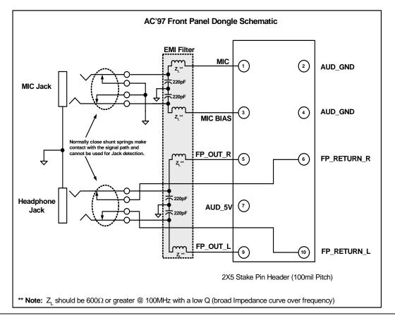
Figure 2. AC'97 Front Panel Dongle Schematic
