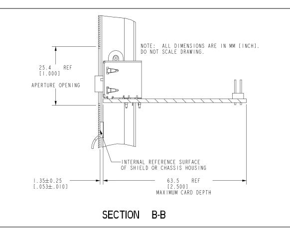
Figure 28. Front Panel I/O Interface Board Placement Recommendations
