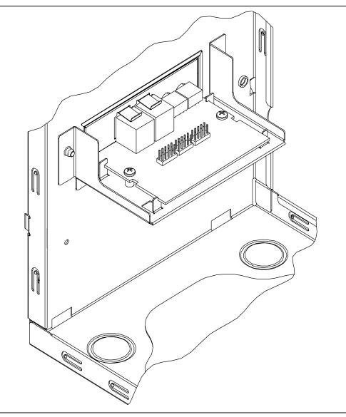
Figure 34. Front Panel I/O Board Support Structure Reference Design
