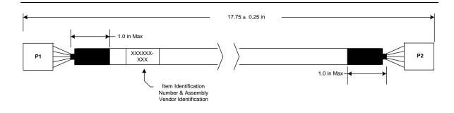
Figure 11. Front Panel Audio Cable Dimensions
