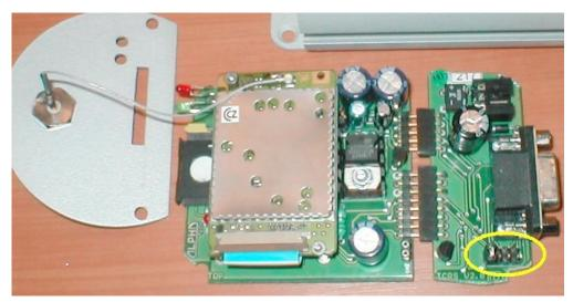
TC35 Alphatech GSM modem: the first jumper from the left is closed.
