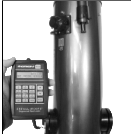
Figure 9. If you stand to the left of the telescope, and face the direction the tube is pointing, the guide arrows will correspond exactly with the direction you should move the telescope in order to find the selected object.
