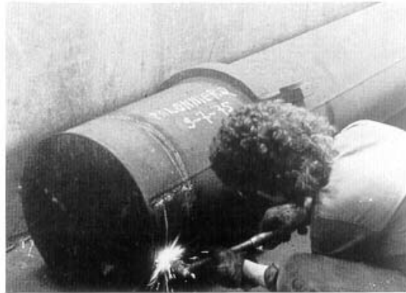
Figure 45: Lifting beam 2 – cutting out of sample
