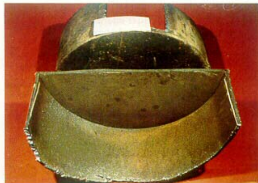
Figure 60: Tube with ends welded to a bottom plate (First inspection programme)
