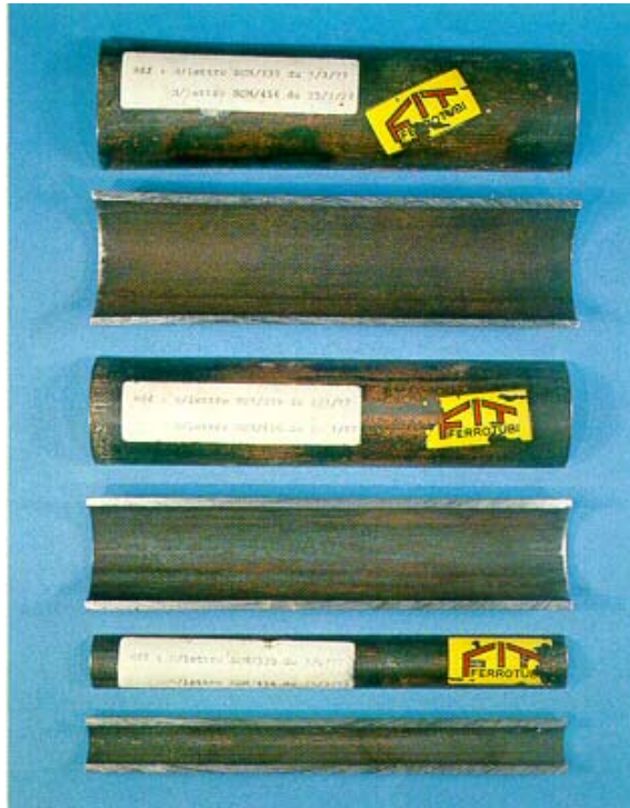
Figure 30 - Internal and external appearance of three samples cut from the tubular framework of an industrial building.
