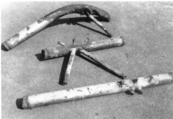
Figure 1: Joint unit with parts of the chords showing severe deformation and rupture at the point of impact.
