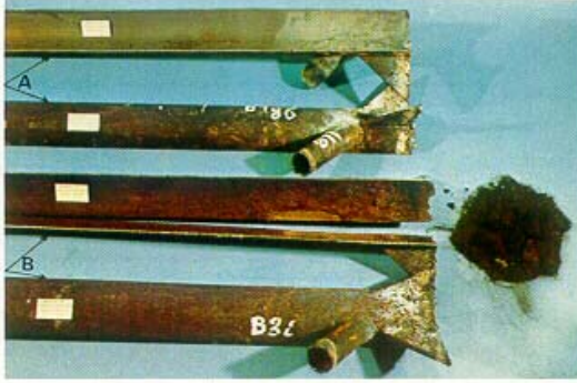
Figure 61: Tube(A) sealed and Tube(B) showing damage going back to original fabrication (First inspection programme)
