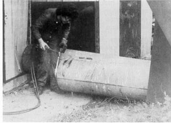
Figure 51: Hall I: single tube semi-portal. Cutting out of the sample
