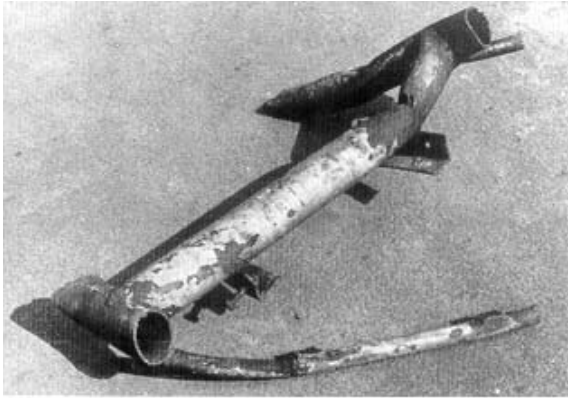
Figure 1: Joint unit with parts of the chords showing severe deformation and rupture at the point of impact.
