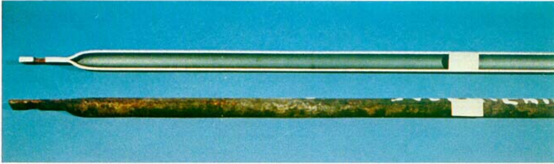
Figure 57: Flattened end tube (First inspection programme)
