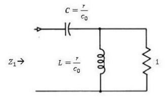
Figure 8: Equivalent circuit of lowest  $TM_{10}$  mode. This is also the equivalent circuit for the radiation given by an infinitesimally small dipole
