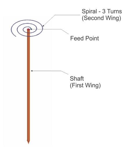
Figure 14: Three turn Spiral Pole
