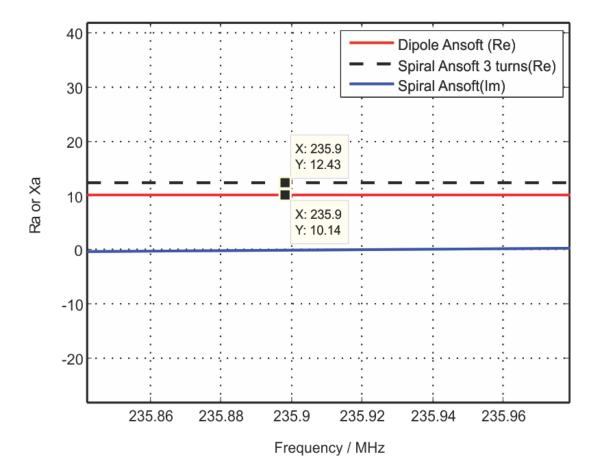
Spiralpole and Dipole Radiation Resistance Comparison
