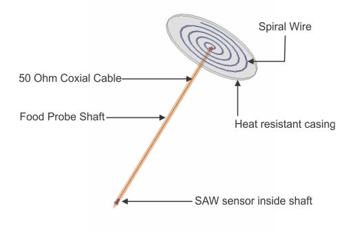
Figure 2: Spiralpole antenna incorporated into wireless food probe design
