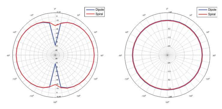
Figure 31: E and H Plane radiation pattern overlays for 5 turn spiralpole and dipole antennas at spiralpole resonance
