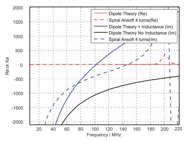
Spiral-pole impedance comparison- Theory vs Simulation
