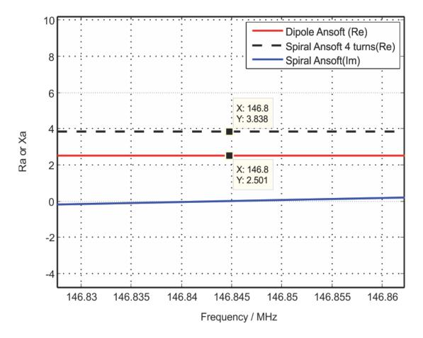
Spiralpole and Dipole Radiation Resistance Comparison
