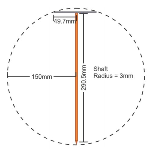
Figure 21: Four turn spiralpole in Chu Sphere
