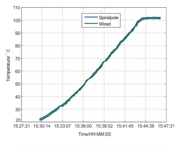
Figure 39: Temperature sensing data acquired with the spiralpole based foodprobe and a wired thermoelement. The spiralpole based wireless solution shows excellent accuracy.
