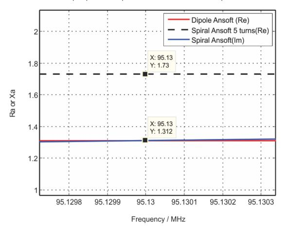
Spiralpole and Dipole Radiation Resistance Comparison
