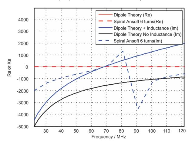
Spiral-pole impedance comparison- Theory vs Simulation
