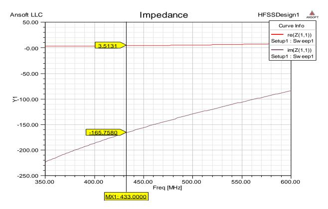
Figure 45: Impedance of disk-dipole hybrid antenna from 350 MHz to 600 MHz. The antenna reactance is primarily capacitive.
