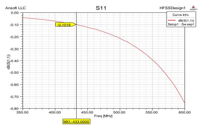
Figure 46: Return Loss (S11) in dB from 350 MHz to 600 MHz of the disk-dipole hybrid. The antenna is starting to resonate at higher frequencies.
