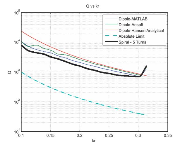
Figure 30: Q - kr for 5 turn spiral VS dipole and absolute limit
