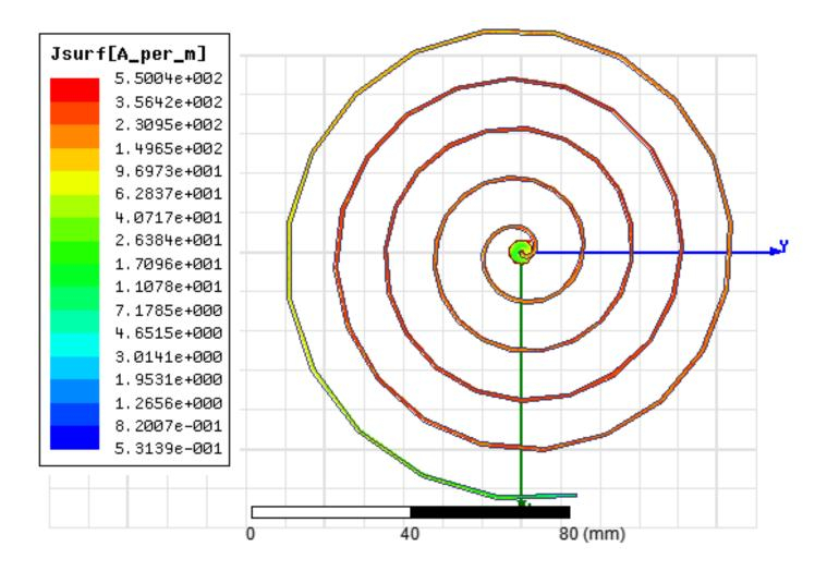
Figure 3: Current distribution at 96MHz (resonance) on a five turns Spiral
