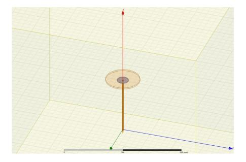
Figure 44: Initial disk-dipole hybrid design in Ansoft\ANSYS HFSS.
