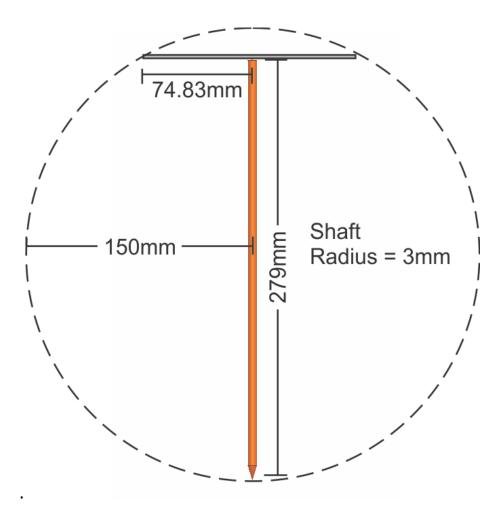
Figure 33: Six turns spiralpole in Chu Sphere
