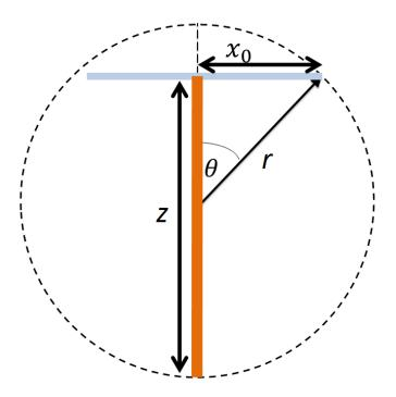
Figure 5: Cross section of a given spiralpole configuration in its minimum bounding sphere
