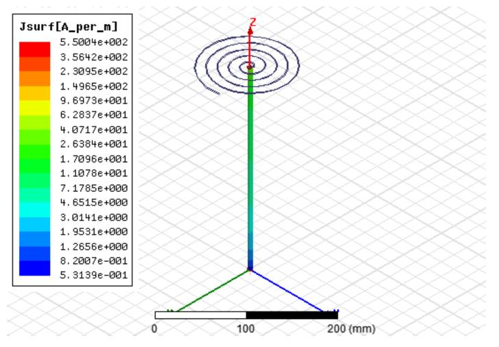
Figure 4: Current distribution on the shaft of the same five turns spiralpole at 96MHz (resonance)
