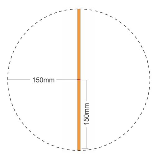
Figure 13: Dipole of length 300mm inside enclosing sphere
