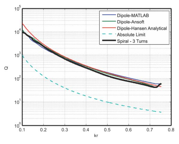
Figure 18: Q - kr for 3 turn spiral VS dipole and absolute limit
