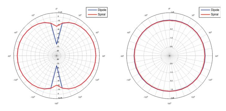
Figure 25: E and H Plane Pattern for 4 turn spiralpole and Dipole at spiralpole resonance
