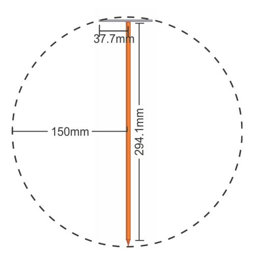
Figure 15: Three turn spiralpole in Chu Sphere
