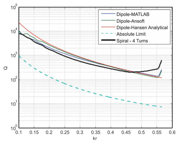
Figure 24: Q - kr for 4 turn spiral VS dipole and absolute limit
