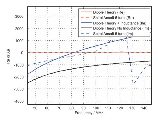
Figure 28: Simulated VS analytical Dipole and 5 turns spiralpole impedances
