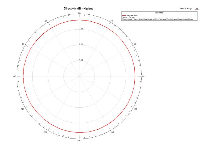
Figure 41: Radiation Pattern in the H plane at 600 MHz. Notice the symmetrical results obtained
