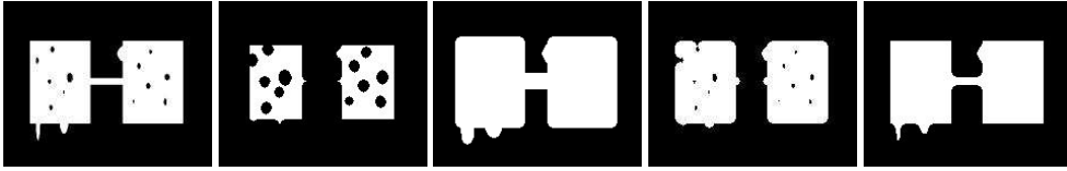
Figure 6.10: The effects of morphological operations on a binary image using a circular structuring element of size 4. From left to right are the original image, erosion, dilation, opening, and closing. The opening operation is erosion of the image followed by dilation. Closing is dilation of the image followed by erosion.
