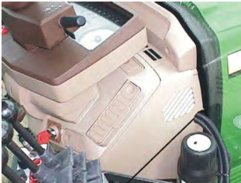
CUT SLOT IN PANEL FOR WIRES FROM SWITCH BOX TO ENTER STEERING COLUMN
