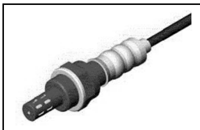
Figure 3-102. Heated Exhaust Gas Oxygen Sensor
