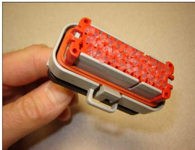
Figure 7-7. Dielectric Grease On Female Contacts
