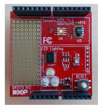
Figure 21: Lighting/Sensor Expansion Board
