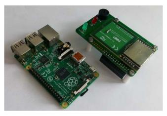
Figure 26: NFC Controller and Raspberry Pi Boards
