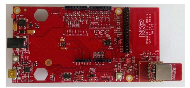
Figure 15: Carrier Board (with a JN5179 Module)
