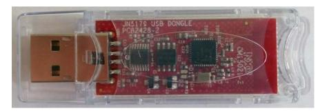
Figure 24: JN5179 USB Dongle
