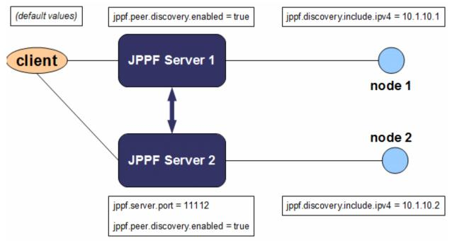
As we can see, automatic discovery involves very few configuration properties. The discovery itself is active by default (jppf.discovery.enabled = true). The client actually does not need any property at all and will work with an empty configuration. The drivers only need to override properties that define non-default values. Lastly, the nodes specify an inclusive pattern for which server to connect to, otherwise they could pickup the wrong server, connect both to the same
