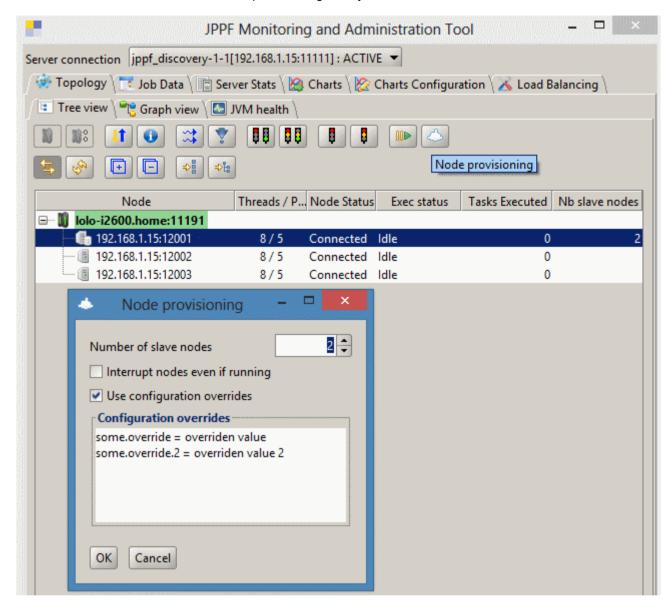
As you can see in this screenshot, the provisioning facility is integrated in the JPPF administration tool. To perform a provisioning operation, in the topology tree or graph view, select any number of master nodes, then click on the provisioning button in the tool bar or in the mouse popup menu.
