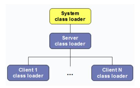
The system class loader is used to start the JPPF node. With most JVMs, it will be an instance of the class java.net.URLClassloader and its usage and creation are handled by the JVM.
