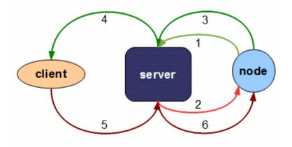
Here, the first two steps are initiated by the server class loader, as a result of the client class loader delegating to its parent. What is missing from this picture are the calls to the system class loader, since they are only meaningful if the requested class is in the node's local classpath.
