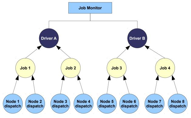
Note that a JPPF job can be submitted to multiple drivers, either in parallel from the same client, or from one driver to another in a multi-driver topology. <u>JobMonitor</u> provides an API to retrieve all the drivers a job is submitted to.
