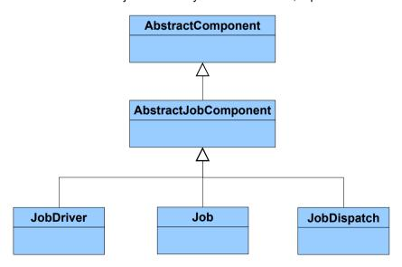
As we can see, job elements share a common super class with the toplogy elements: AbstractComponent, which provides the base API to navigate a tree of elements identified by their uuid.
