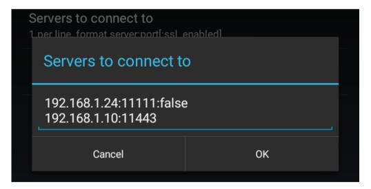
The node will try all the defined servers in order, until it establishes a connection. When all servers have been tried, it will start back from the first in the list. The format of a connection definition is as follows:
