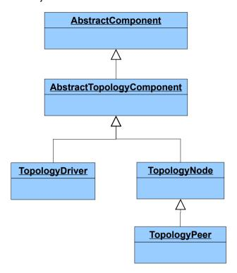
AbstractComponent provides the API to navigate a tree of elements uniquely identified with a uuid:
