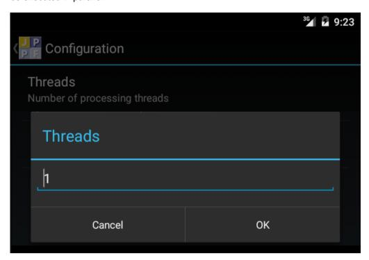
This is equivalent to setting the configuration property "jppf.processing.threads" in a standard JPPF node.
