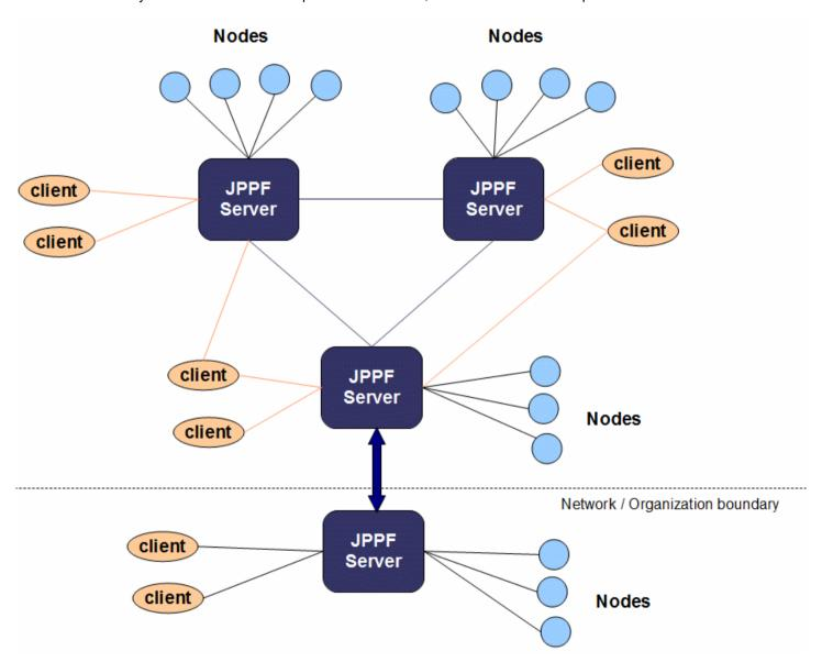
The role of the configuration will be essentially to determine where each component can find the others, and how their interactions will be processed.
