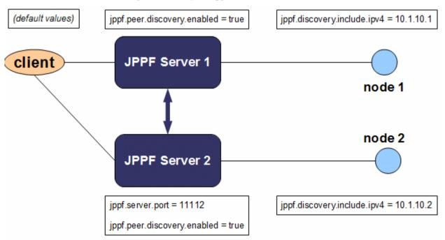
As we can see, automatic discovery involves very few configuration properties. The discovery itself is active by default (jppf.discovery.enabled = true). The client actually does not need any property at all and will work with an empty configuration. The drivers only need to override properties that define non-default values. Lastly, the nodes specify an inclusive pattern for which server to connect to, otherwise they could pickup the wrong server, connect both to the same
