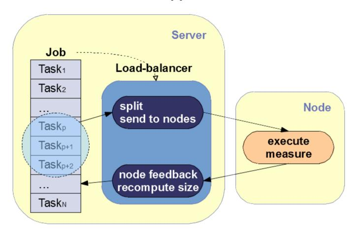
As we can see, from a high-level perspective it is made of a continuous feedback loop:
