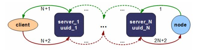
It is also important to note that this does not change anything to the class loader hierarchy within the node. In effect, there is still only one server class loader, which is associated with the server the node is *directly* connected to. This implies that the parent delegation model will not cause a class loading request to traverse the server chain multiple times.
