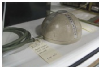
Figure 0.14 The first computer mouse. https://commons.wikimedia.org/wiki/File:Telefunken_Rollkugel_RKS_100-86.jpg
