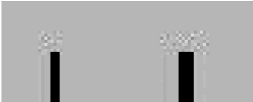
Figure 8.1 JPEG images tend to show artifacts at places where pixels change rapidly, like corners and edges.
