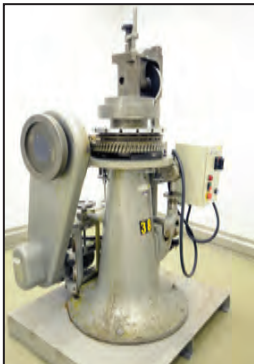
MANESTY D3B 16 station rotary tablet press
