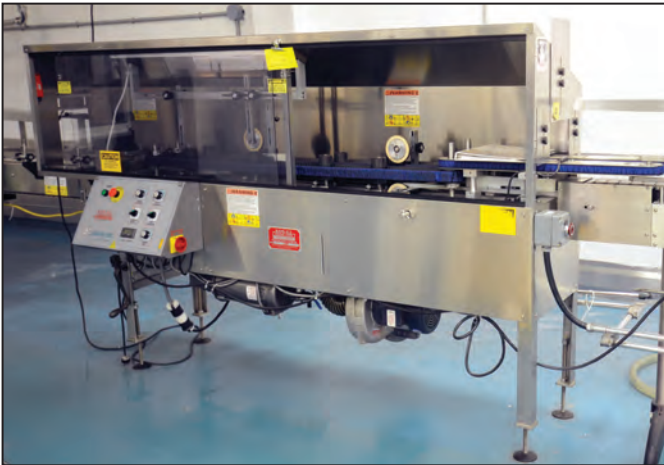
KAPS-ALL CLEAN-N-VAC AC1 container cleaner
