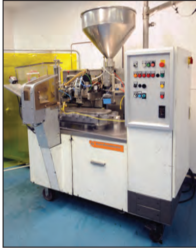
NORDEN NM620 HA/M hot air automatic plastic tube filler
