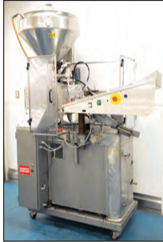
KALIX KX60 rotary tube filler/sealer
