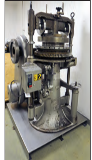
MANESTY BB3B 27 station rotary tablet press
