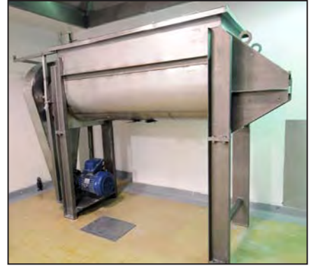
AARON 22 cu/ft stainless steel double ribbon blender
