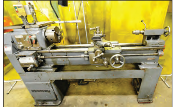
MYSORE 14" X 40" tool room lathe
