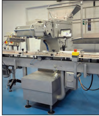
CREMER TO1220 12 lane, tablet & capsule counter & filler
