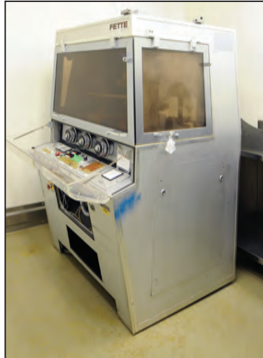
FETTE P1000 22 station rotary tablet press
