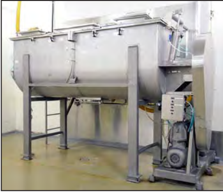
96 cu/ft stainless steel double ribbon blender
