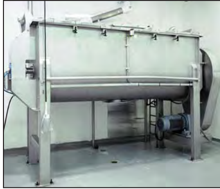
96 cu/ft stainless steel double ribbon blender
