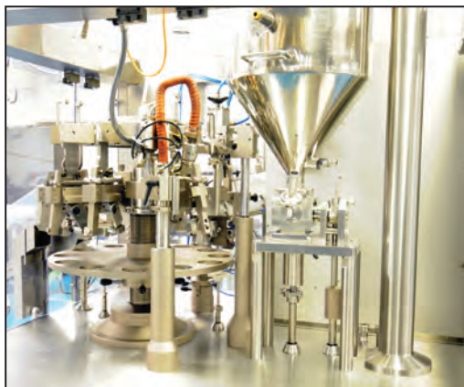
ROMACO UNIPAC U 20100 12-station high speed single nozzle modular automatic tube filler and sealer
