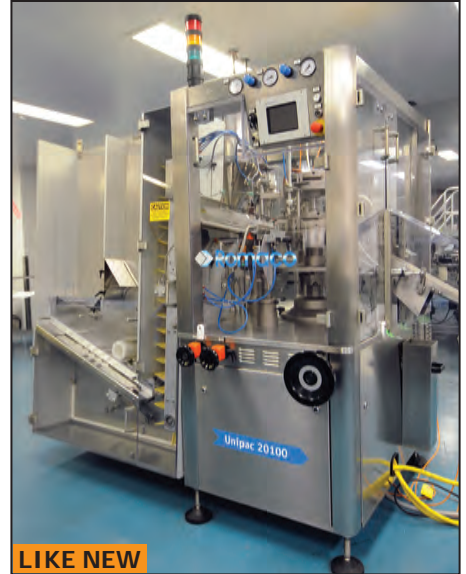
ROMACO UNIPAC U 20100 12-station high speed single nozzle modular automatic tube filler & sealer
