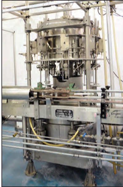
HORIX HBX-9 9 head rotary liquid filler
