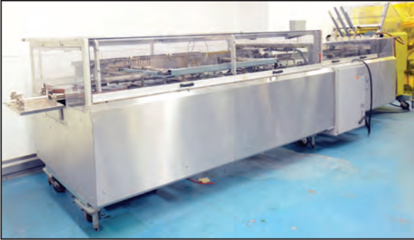
RA JONES IMV semi automatic, intermittent motion, vertical cartoner
