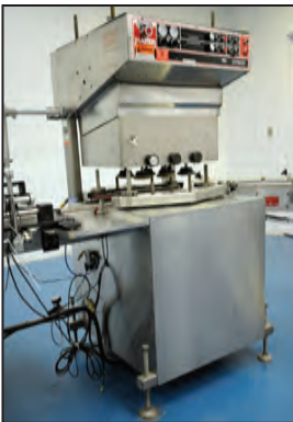
FAIRCHILD CAPMASTER 6 spindle cap torque
