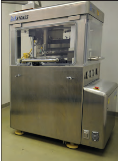
STOKES 571S GEM SUPREME 34 station rotary tablet press
