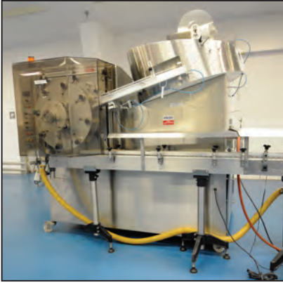
KALISH 7420 KALISHSORT bottle unscrambler w/ feed elevator
