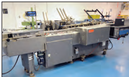
BOSCH CORTINA 200 horizontal continuous motion cartoner
