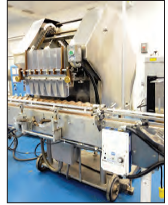
LAKSO 93 slit type tablet & capsule counter & filler
