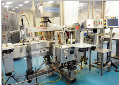
NEW JERSEY 305SR-1447 front & back pressure sensitive labeller
