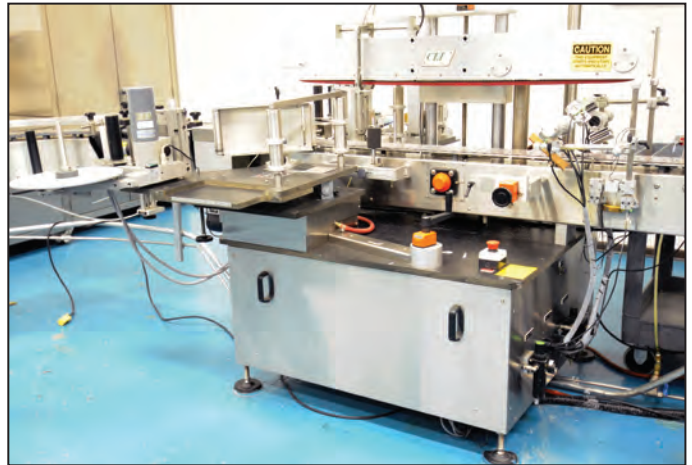
CLI UNI 510 wraparound pressure sensitive labeller
