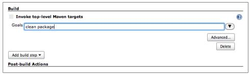
Figure 2-17. Adding a build step
