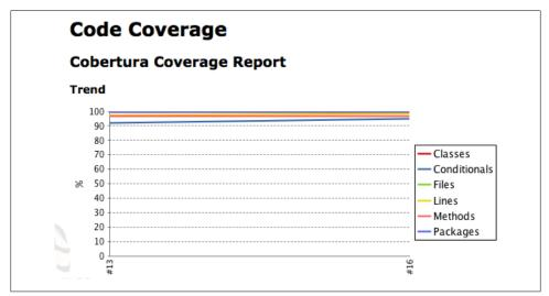
Figure 2-32. Jenkins also displays a graph of code coverage over time
