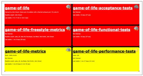
Figure 8-8. Displaying a build radiator view
