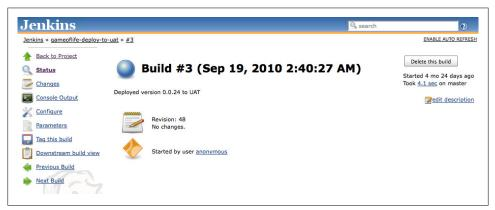
Figure 10-14. Jenkins stores what parameter values where used for each build
