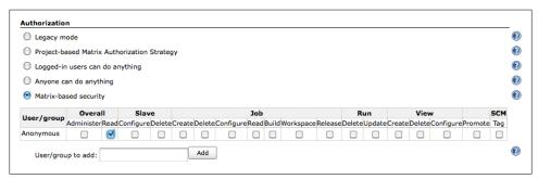
Figure 7-16. Matrix-based security configuration
