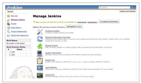
Figure 3-10. Upgrading Jenkins from the web interface
