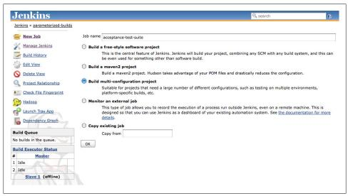
Figure 10-19. Creating a multiconfiguration build job
