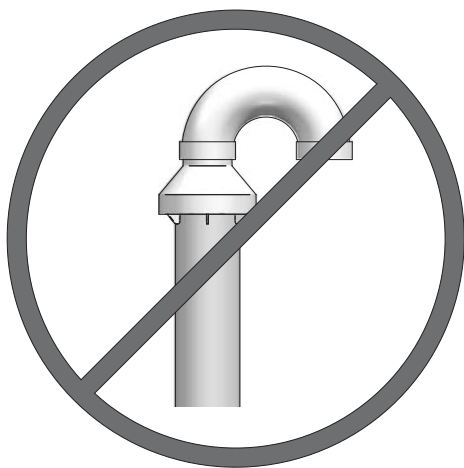
Figure 5-5 Do Not Install U-Bent to Rain Cap
