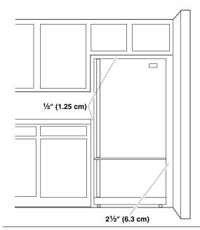
To ensure proper ventilation for your refrigerator, allow for  $\frac{1}{2}$  (1.25 cm) space on each side and at the top. Allow at least 1" (2.54 cm) between the back of the cabinet and the wall. If your refrigerator has an ice maker, make sure you leave extra space at the back for the water line connections.
