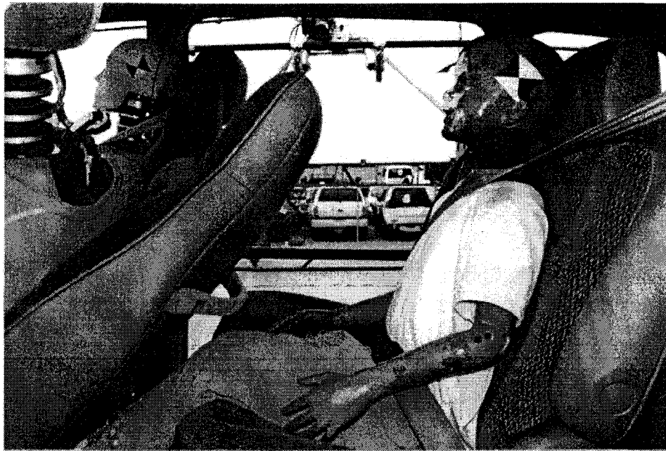
Figure 7. Close Up Showing Head Strike and Leg Impact Chalk Marks on Rear Child
